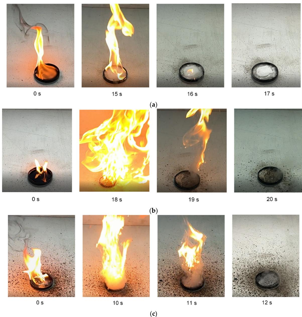
**Figure 4.** Images of flammable liquid fire suppression ( $V_0 \approx 3 \text{ mL}$ ) by carbon dioxide hydrate powder,  $m_g \approx 4 \text{ g}$ : (a) kerosene; (b) motor oil; (c) crude oil ( $d_f \approx 65 \text{ mm}$ ,  $S_f \approx 33 \text{ cm}^2$ ).
