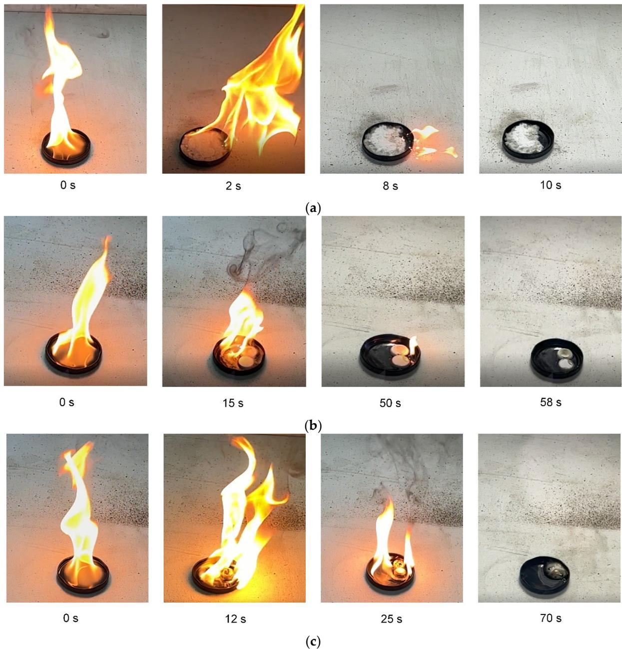
**Figure 2.** Images of gasoline fire suppression ( $V_0 \approx 3$  mL) with the help of carbon dioxide hydrate in the forms of (a) powder,  $m_g \approx 4$  g; (b) tablets,  $m_g \approx 1.07$  g; (c) spheres,  $m_g \approx 1.42$  g ( $d_f \approx 65$  mm,  $S_f \approx 33$  cm<sup>2</sup>).
