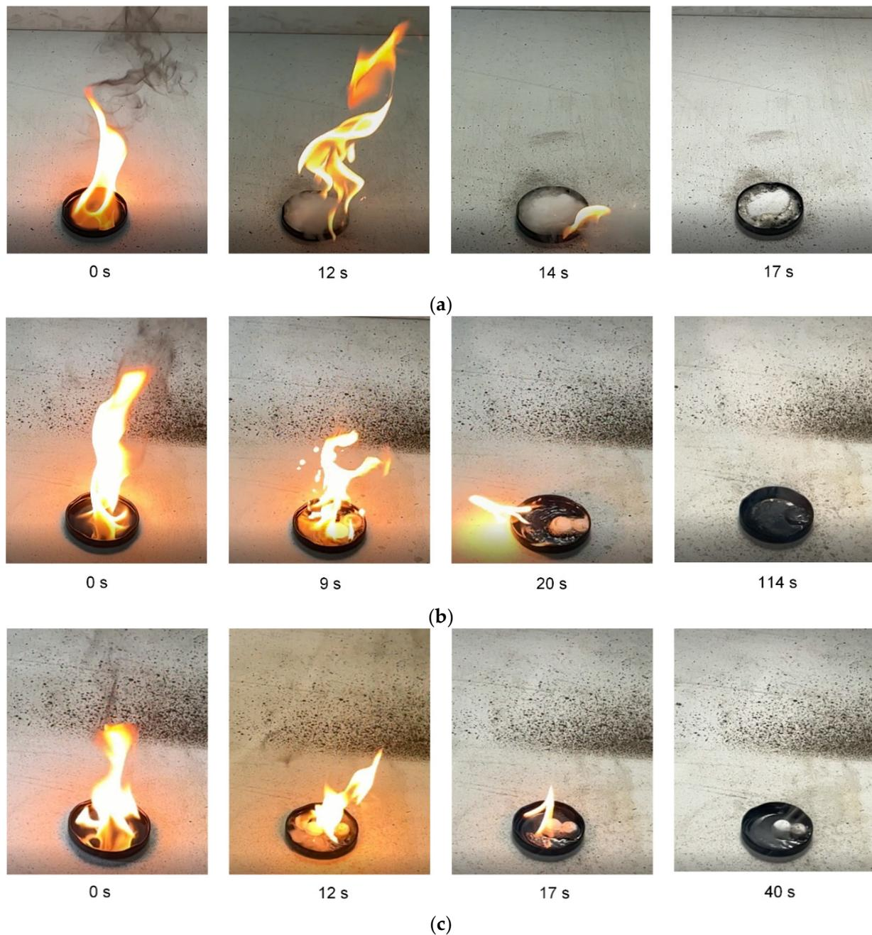
**Figure 3.** Images of Diesel fuel fire suppression ( $V_0 \approx 3$  mL) with the help of carbon dioxide hydrate in the forms of (a) powder,  $m_g \approx 4$  g; (b) tablets,  $m_g \approx 1.07$  g; (c) spheres,  $m_g \approx 1.42$  g ( $d_f \approx 65$  mm,  $S_f \approx 33$  cm<sup>2</sup>).
