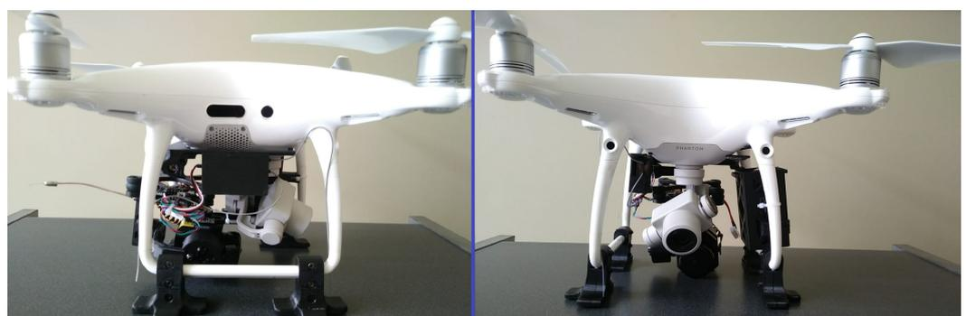
**Figure 6.** Side (left) and front (right) view of the UAV with infrared and RGB cameras used in the investigation.
