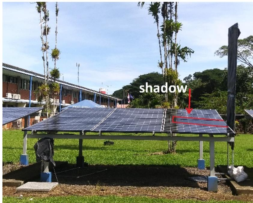
**Figure 7.** Object used to generate partial shade conditions. The shadow generated corresponds to the PS1 suboptimal condition.
