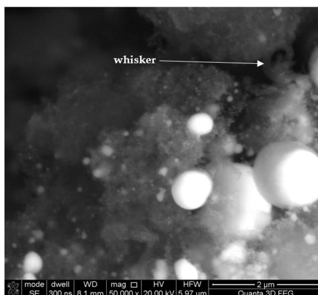
Figure 7. SEM image of the surface of the used catalyst. Magnification  $\times 50,000$ . Power—25 W. Temperature—500 °C.
