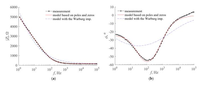
**Figure 10.** Measurement and approximating frequency characteristics of: (**a**) modulus and (**b**) argument of impedance of a symmetrical supercapacitor with collectors containing polypyrrole, containing LiClO<sub>4</sub> as an active electrolyte component.
