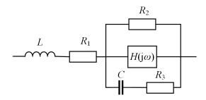
Figure 3. Fractional-order supercapacitor topology using the Havriliak–Negami function.
