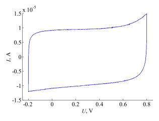
**Figure 7.** Cyclic voltammogram of the symmetric supercapacitor containing LiClO<sub>4</sub> as the active electrolyte component, with collectors containing polypyrrole.
