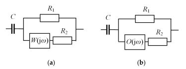
**Figure 2.** Topologies of fractional-order supercapacitor models: (**a**) four-parameter structure with Warburg impedance, (**b**) five-parameter structure with limited Warburg impedance.
