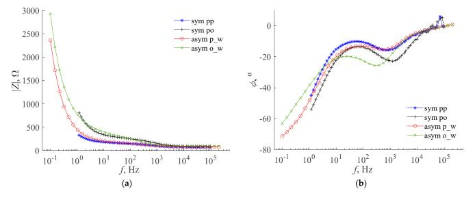
**Figure 9.** Measurement frequency characteristics of: (a) modulus and (b) argument of impedance of the tested symmetric supercapacitors containing  $NBu_4ClO_4$  as the active electrolyte component.
