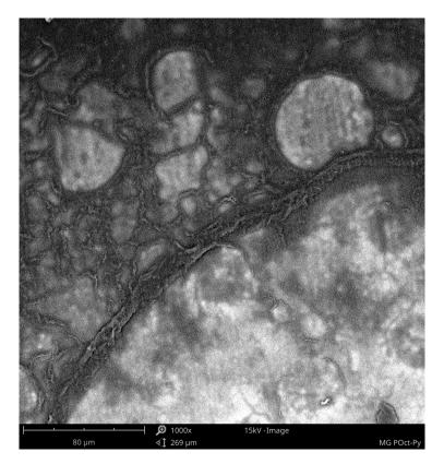
**Figure 6.** SEM photo of a poly(3-n-octylopyrrole), zoom  $\times 1000$ .
