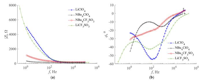
**Figure 8.** Measurement frequency characteristics of: (**a**) modulus and (**b**) argument of impedance of the tested symmetric supercapacitors with collectors containing polypyrrole.
