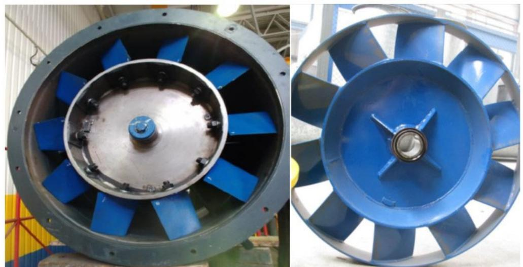
Figure 15. Comparison of the new (left) and datum (right) rotor design.
