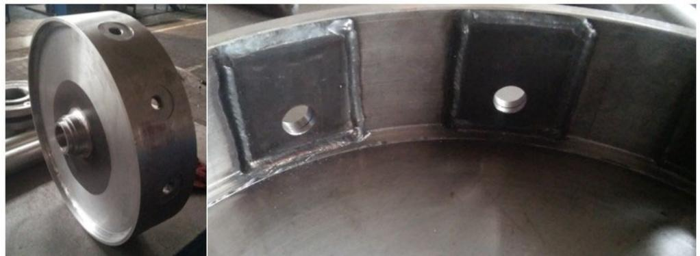
Figure 14. View of the rotor with blades sockets.
