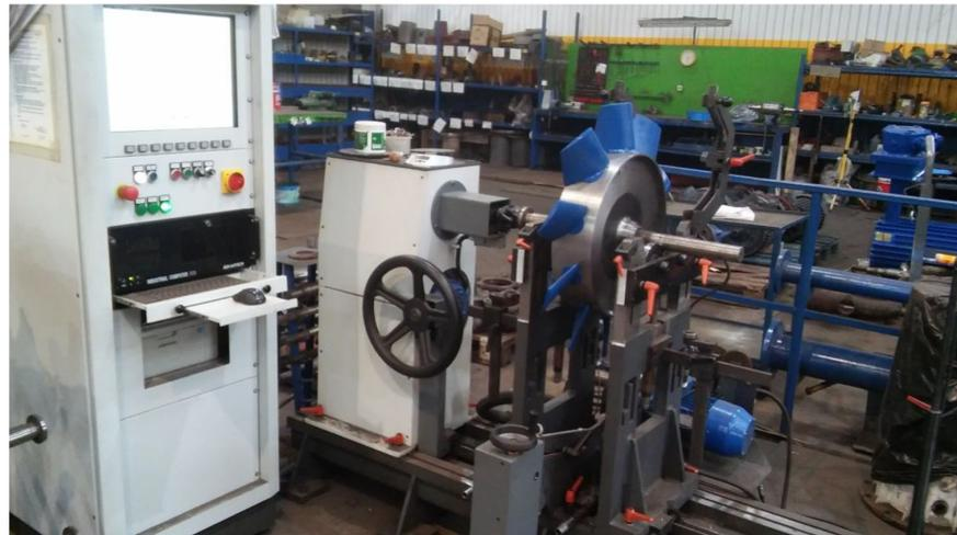
Figure 18. Balancing of the rotor.
