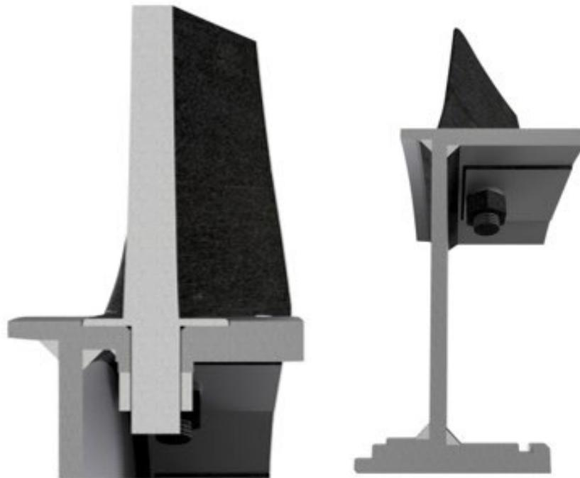
Figure 13. Blade fastening method.
