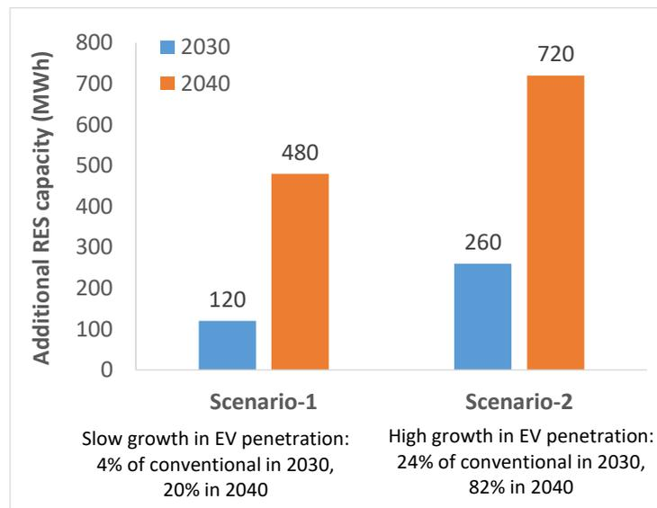
**Figure 11.** Increase in RES hosting capacity in the Greek islands with the application of V2G methodologies [47].
