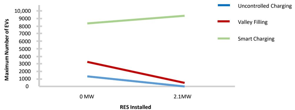
**Figure 12.** Relation between the maximum allowed number of EVs and the RESs installed in the network of Ikaria (based on the results of the Merge EU project) [49].
