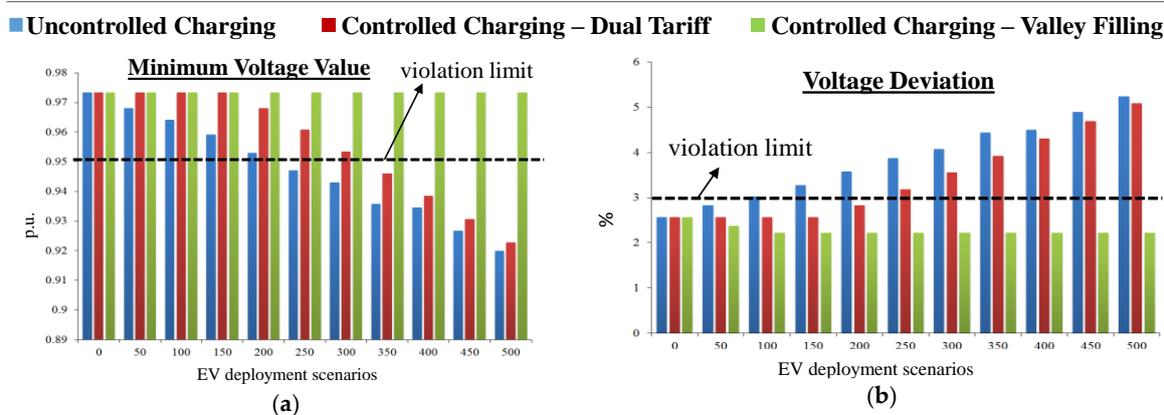
**Figure 9.** Voltage values for various EV penetration scenarios in the island of Ikaria (a 1 MW wind generator is considered to operate in the island for the scenarios examined): (a) minimum voltage value and (b) voltage deviation [48].
