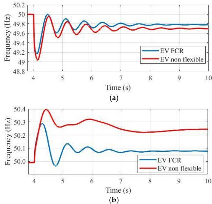
**Figure 5.** Contribution of EV charging in (a) underfrequency and (b) overfrequency transients.
