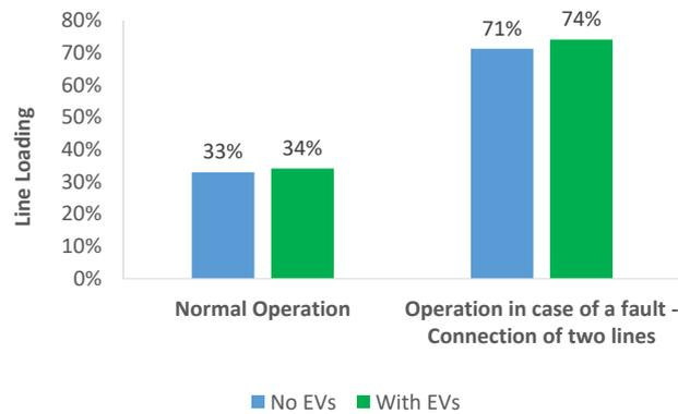
Figure 7. Maximum loading of the lines in Astypalea when considering the presence of EVs.
