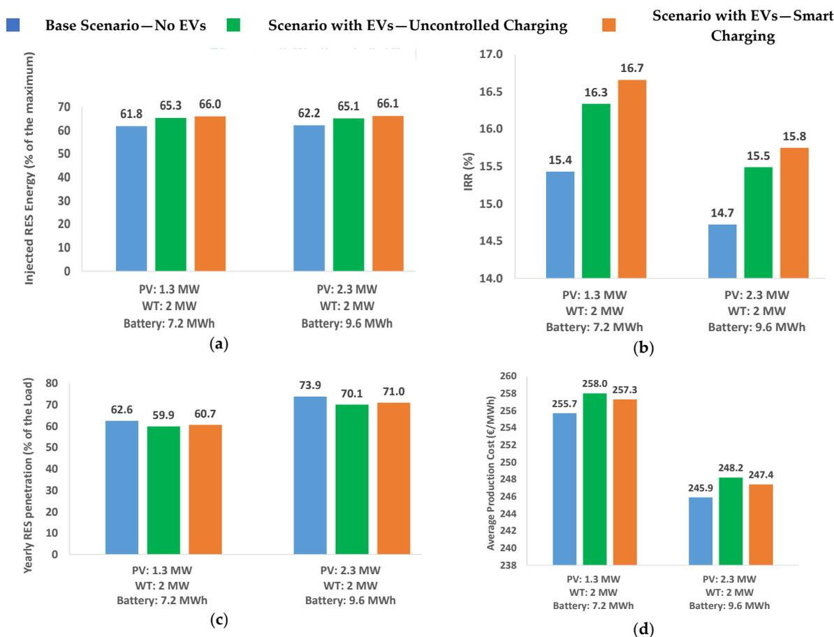
**Figure 4.** The impact of EV charging in Astypalea [45] regarding (a) injected RES energy (% of the maximum available), (b) IRR, (c) RES penetration (% of the system's demand), and (d) average production cost [45].
