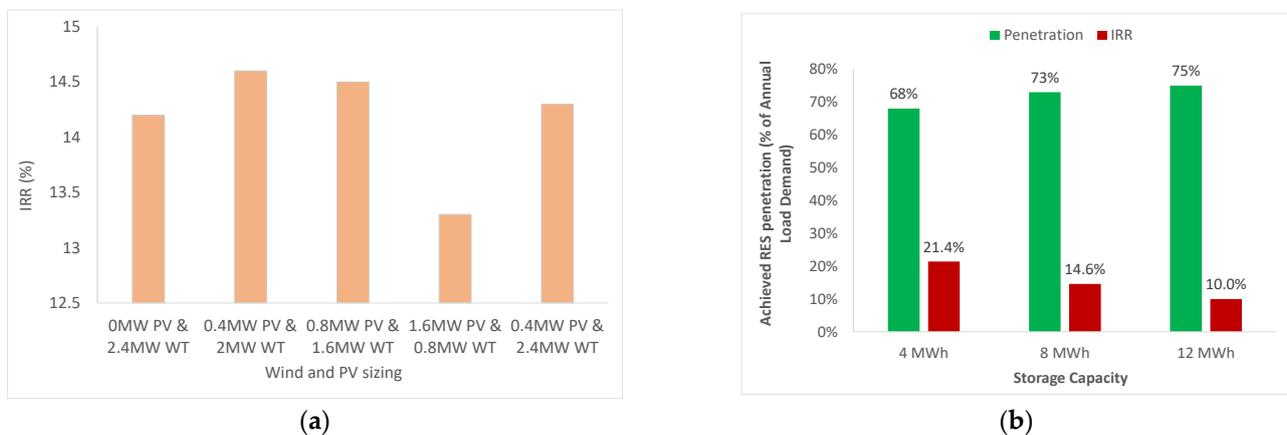
Figure 2. (a) Internal rate of return (IRR) for different RES capacity combinations in Astypalea; (b) IRR and achieved RES penetration for different storage capacities [14].
