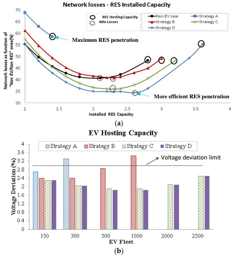
**Figure 10.** (a) Network losses for various cases of RES penetration when considering the introduction of 300 EVs in the island of Ikaria; (b) voltage deviation for various levels of EV penetration when considering that 2.1 MW RESs are installed in the island of Ikaria [37].
