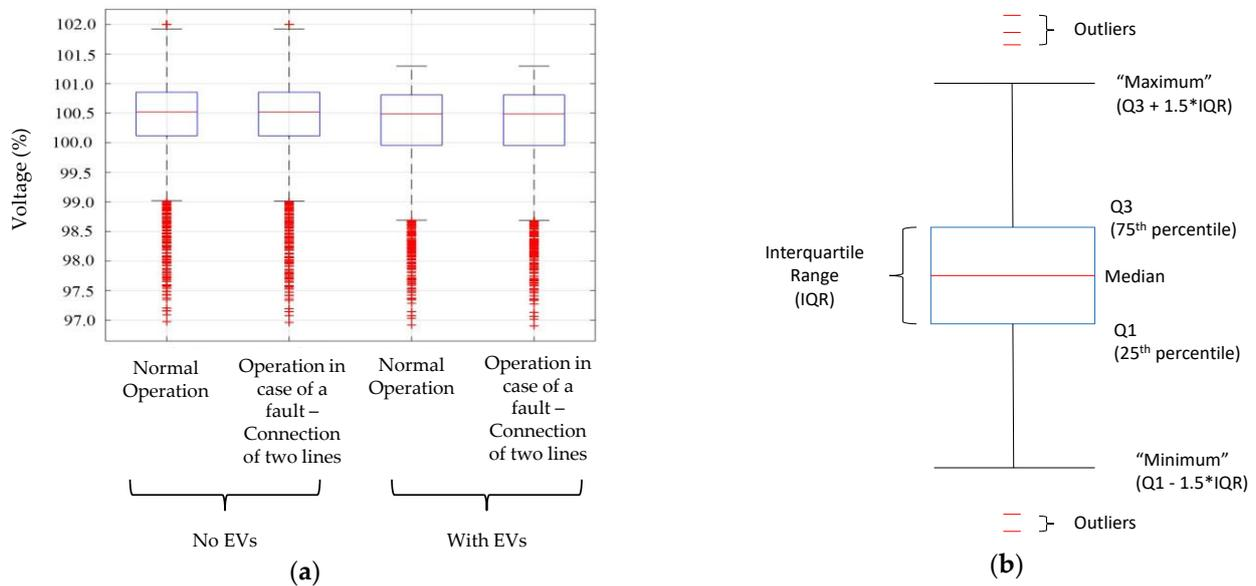
Figure 8. (a) Boxplot for the minimum voltage values in Astypalea when considering the presence of EVs, (b) Explanation of the boxplot.
