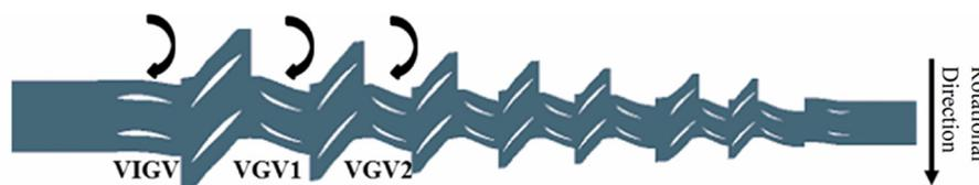
**Figure 2.** Turning direction of VGVs.
