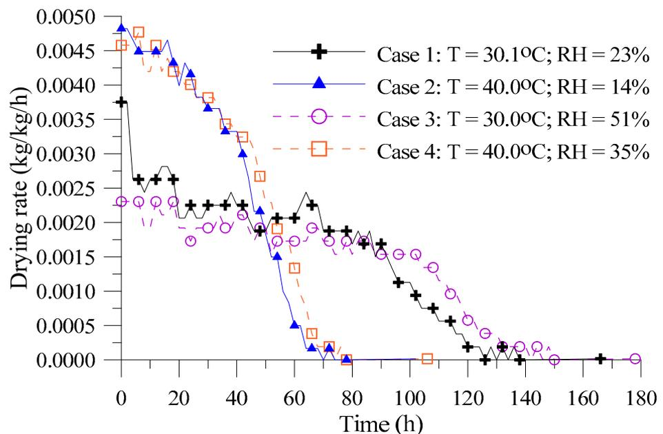
Figure 6. Drying rate of samples as a function of time during drying process.
