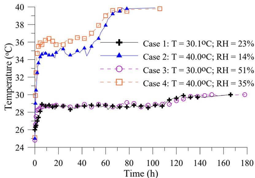
**Figure 9.** Surface temperature of samples as a function of time during drying process.
