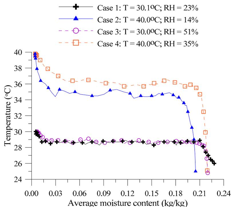
Figure 10. Surface temperature of sample as a function of average moisture content.
