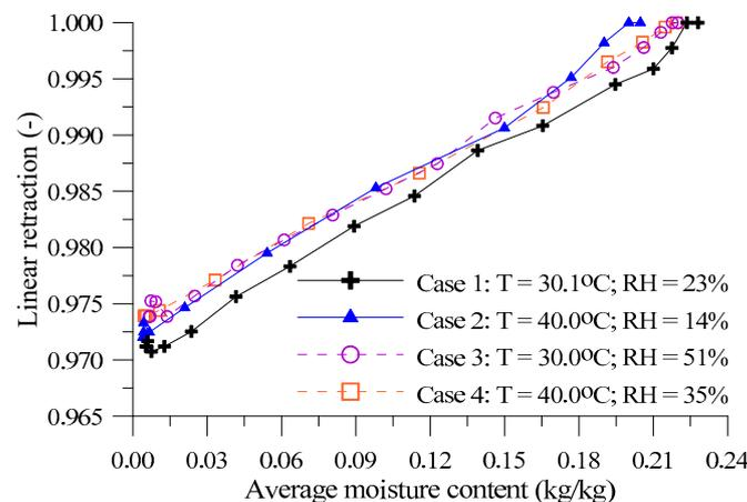
**Figure 13.** Linear retraction of sample as a function of average moisture content during drying process.
