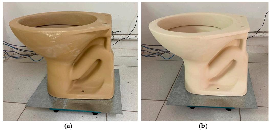
**Figure 8.** Sample used in Case 3 (TECNOMAT laboratory;  $T = 30.0\text{ }^{\circ}\text{C}$ ;  $\text{RH} = 51\%$ ) before (a) and after (b) oven drying experiment.
