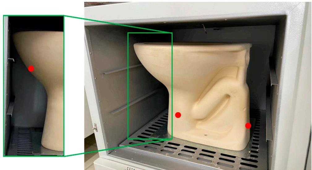
**Figure 3.** Indication of temperature measurement points at sample surface.
