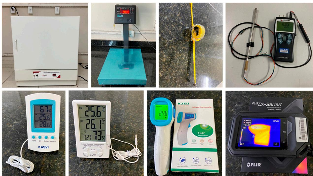
**Figure 2.** Equipment used in drying experiment: oven, digital scale, measuring tape, hot wire anemometer, two thermo-hygrometers, digital infrared thermometer and thermographic camera.
