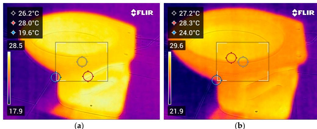
**Figure 11.** Thermograms of sample used in Case 3 ( $T = 30.0\text{ }^{\circ}\text{C}$  and  $\text{RH} = 51\%$ ) for time instants (a)  $t = 36\text{ h}$  and (b)  $t = t_e = 178\text{ h}$ .
