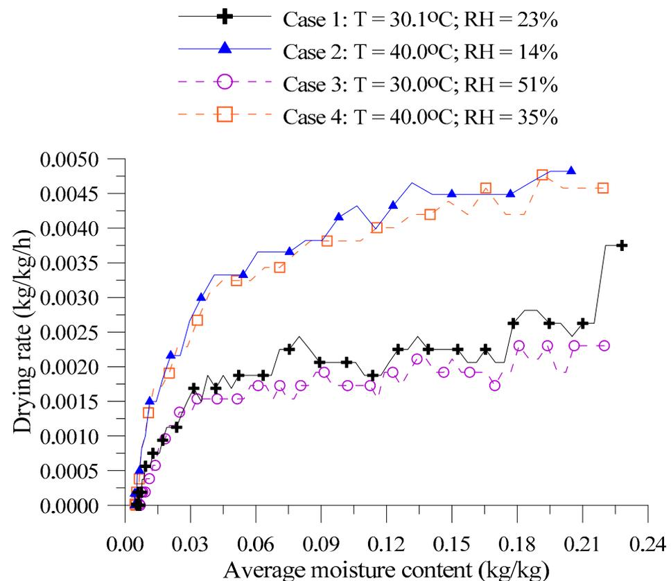
**Figure 7.** Drying rate as a function of average moisture content of samples during drying process.
