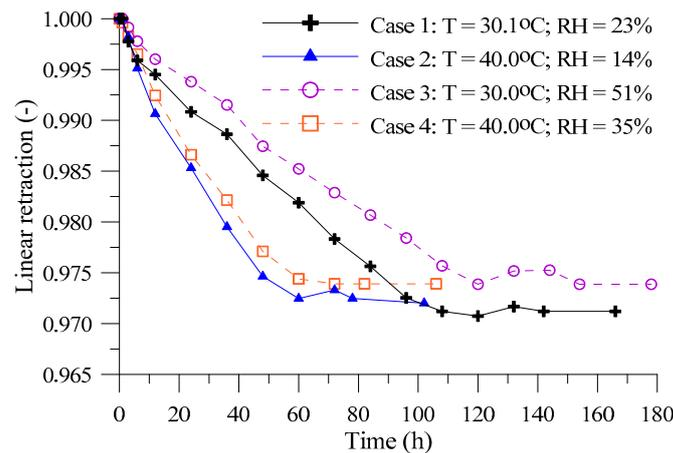
**Figure 12.** Linear retraction of sample as a function of time during drying process.
