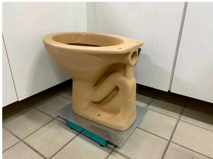
**Figure 1.** Sanitary toilet before drying experiment.
