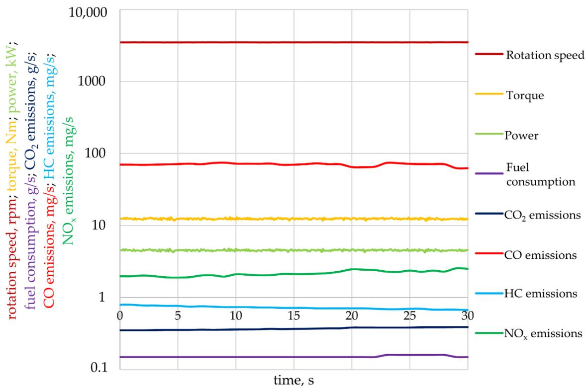
**Figure 3.** Example of characteristics of the tested parameters as a function of time for fan W1 during open flow measurement (Method B).
