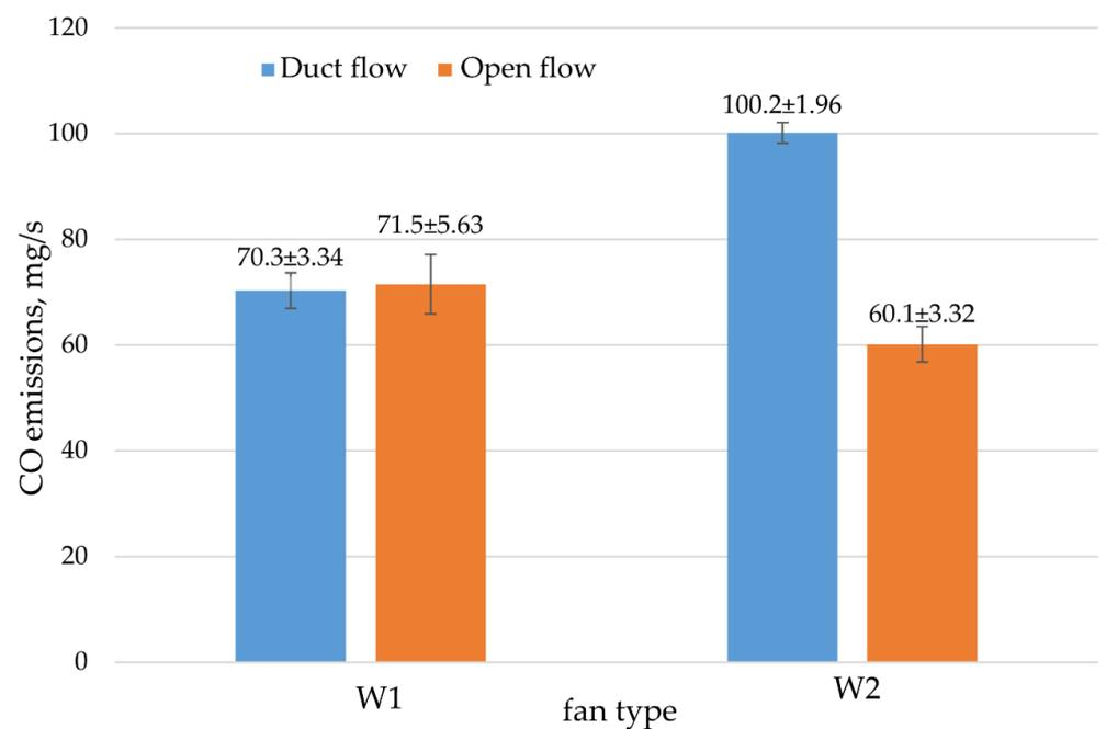
**Figure 9.** Mean CO emissions during tests with Methods A (duct flow) and B (open flow), where W1—fan with conventional impeller, W2—fan with turbo impeller. All mean values were determined at a 95% confidence interval ( $p = 0.05$ ).
