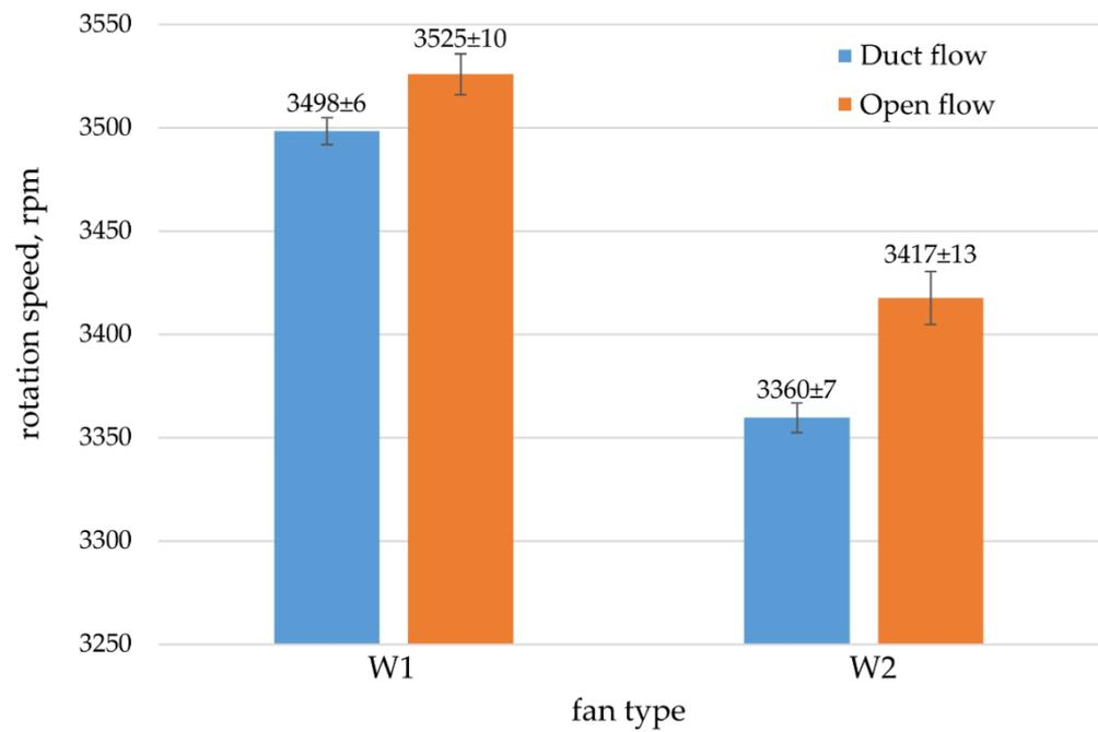
**Figure 4.** Mean speed during tests with Methods A (duct flow) and B (open flow), where W1—fan with conventional impeller, W2—fan with turbo impeller. All mean values were determined at a 95% confidence interval ( $p = 0.05$ ).
