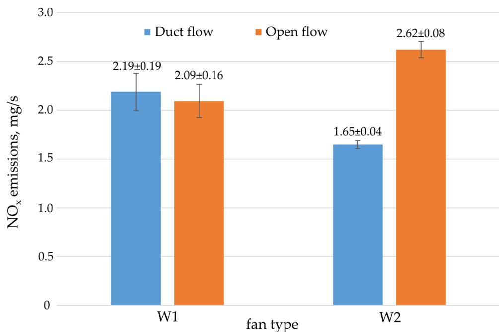
**Figure 11.** Mean NO<sub>x</sub> emissions during tests with Methods A (duct flow) and B (open flow), where W1—fan with conventional impeller, W2—fan with turbo impeller. All mean values were determined at a 95% confidence interval ( $p = 0.05$ ).
