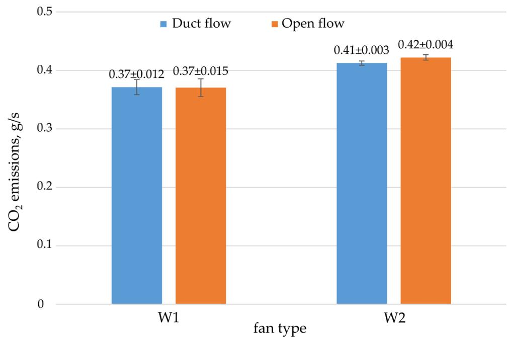
**Figure 8.** Mean CO<sub>2</sub> emissions during tests with Methods A (duct flow) and B (open flow), where W1—fan with conventional impeller, W2—fan with turbo impeller. All mean values were determined at a 95% confidence interval ( $p = 0.05$ ).
