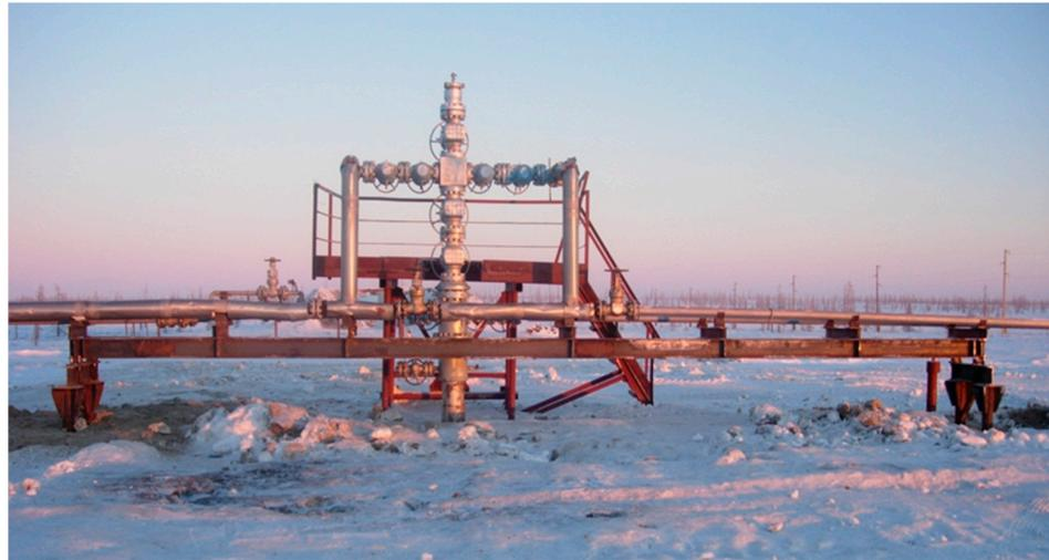
**Figure 15.** Strengthening the wellhead by long steel beam in unstable permafrost [16].
