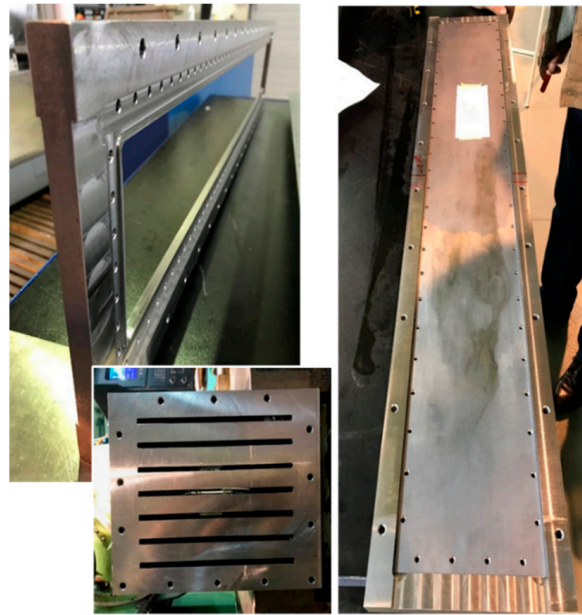
Figure 8. Modular PAV prototype made of vanadium.
