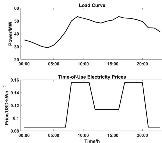
**Figure 1.** Typical daily load curve and time-of-use electricity prices.
