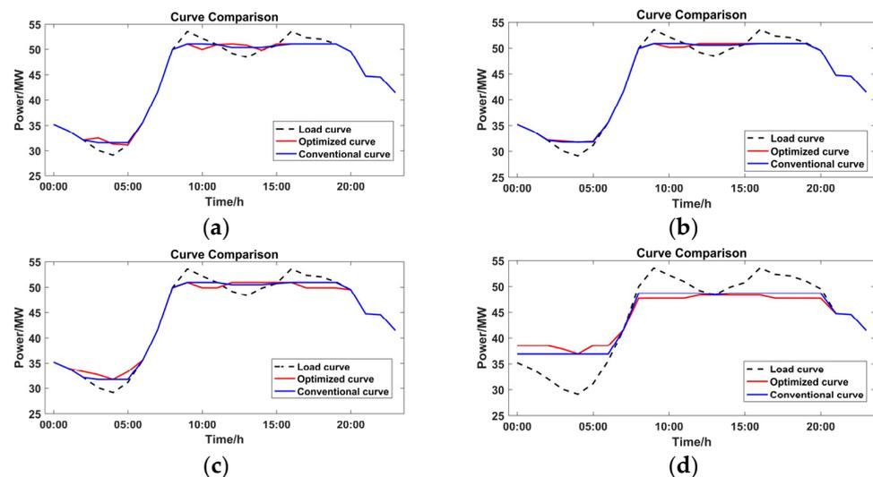
Figure 4. Comparison of load curves after the participation of energy storage: (a)  $\beta = 0$ ; (b)  $\beta = 1000$ ; (c)  $\beta = 5000$ ; (d)  $\beta = 10,000$ .
