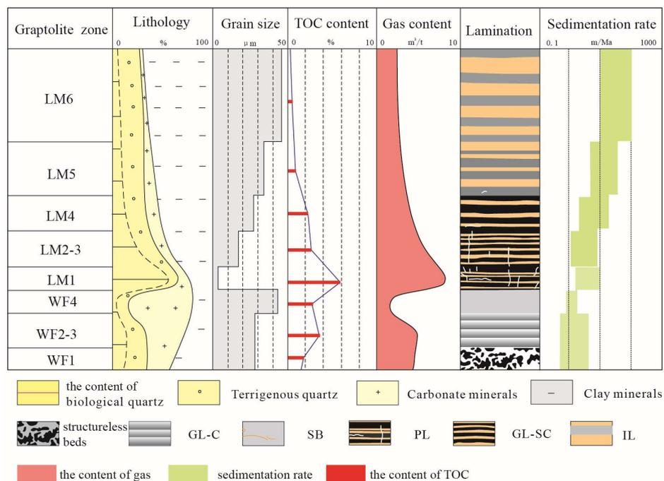
Figure 5. The parameters of shale gas in Longmaxi Formation. Reprint with permission from Ref. [14]. 2022, Zhensheng Shi.
