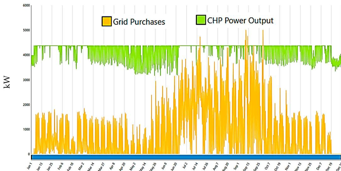
Figure 7. Output power (System 1: grid and CHP).
