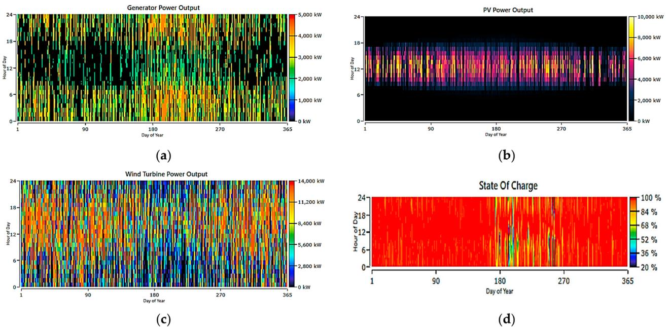
Figure 23. System 6: CHP, PV, ESS, and wind (a) CHP output power, (d) PV power output, (c) wind output power, and (d) state of charge.
