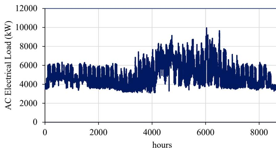
Figure 3. Load profile for OU “from facility management department”.
