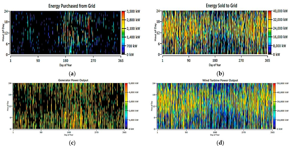
Figure 17. System 4: grid, CHP, and wind, (a) energy purchased from grid, (b) energy sold to grid, (c) CHP output power, and (d) wind power output.
