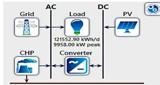
Figure 9. System 2: grid, CHP, and PV design.
