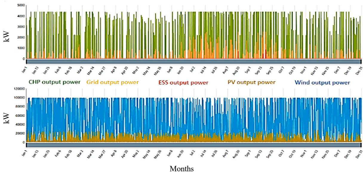
Figure 19. Output power (System 5: grid, CHP, PV, ESS, and wind).
