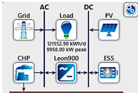
Figure 12. System 3: grid, CHP PV, and ESS design.
