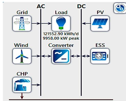
Figure 18. System 5: grid, CHP, wind, PV, and ESS design.
