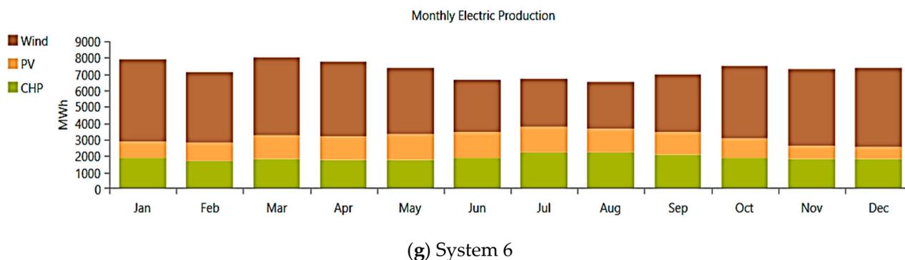
**Figure 24.** Monthly electric production for all proposed systems.
