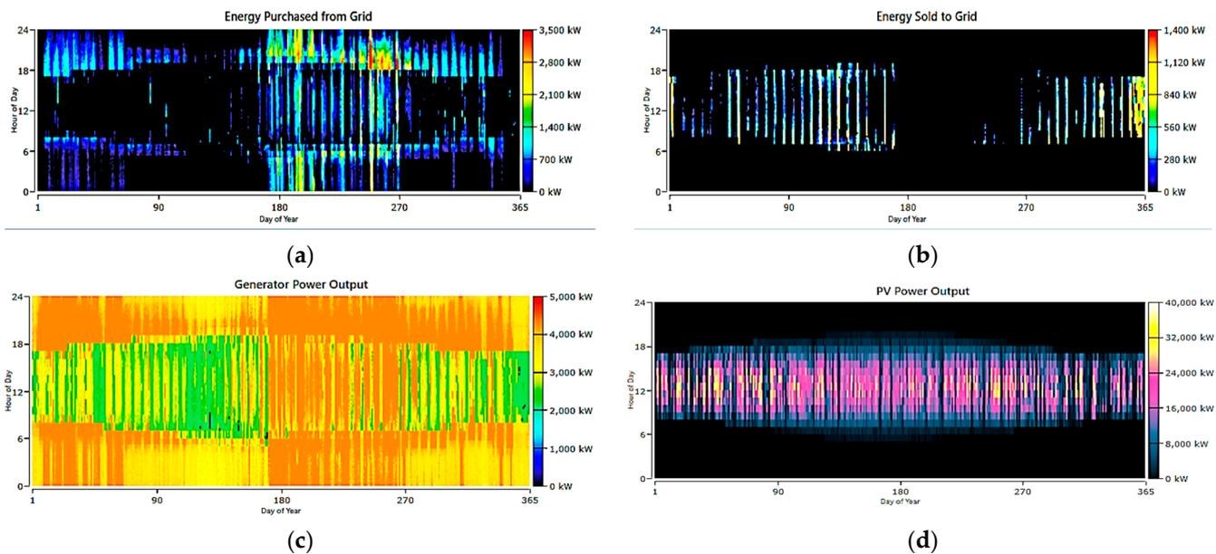
Figure 11. System 2: grid, CHP, and PV (a) energy purchased from grid, (b) energy sold to grid, (c) CHP output power, and (d) PV power output.
