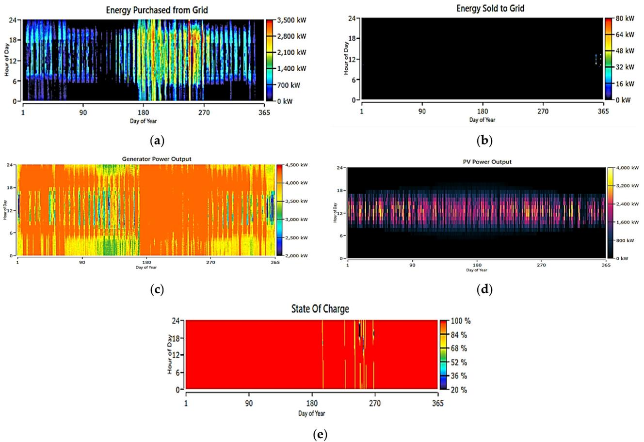
**Figure 14.** System 3: grid, CHP, PV, and ESS (a) energy purchased from grid, (b) energy sold to grid, (c) CHP output power, (d) PV power output, and (e) state of charge.
