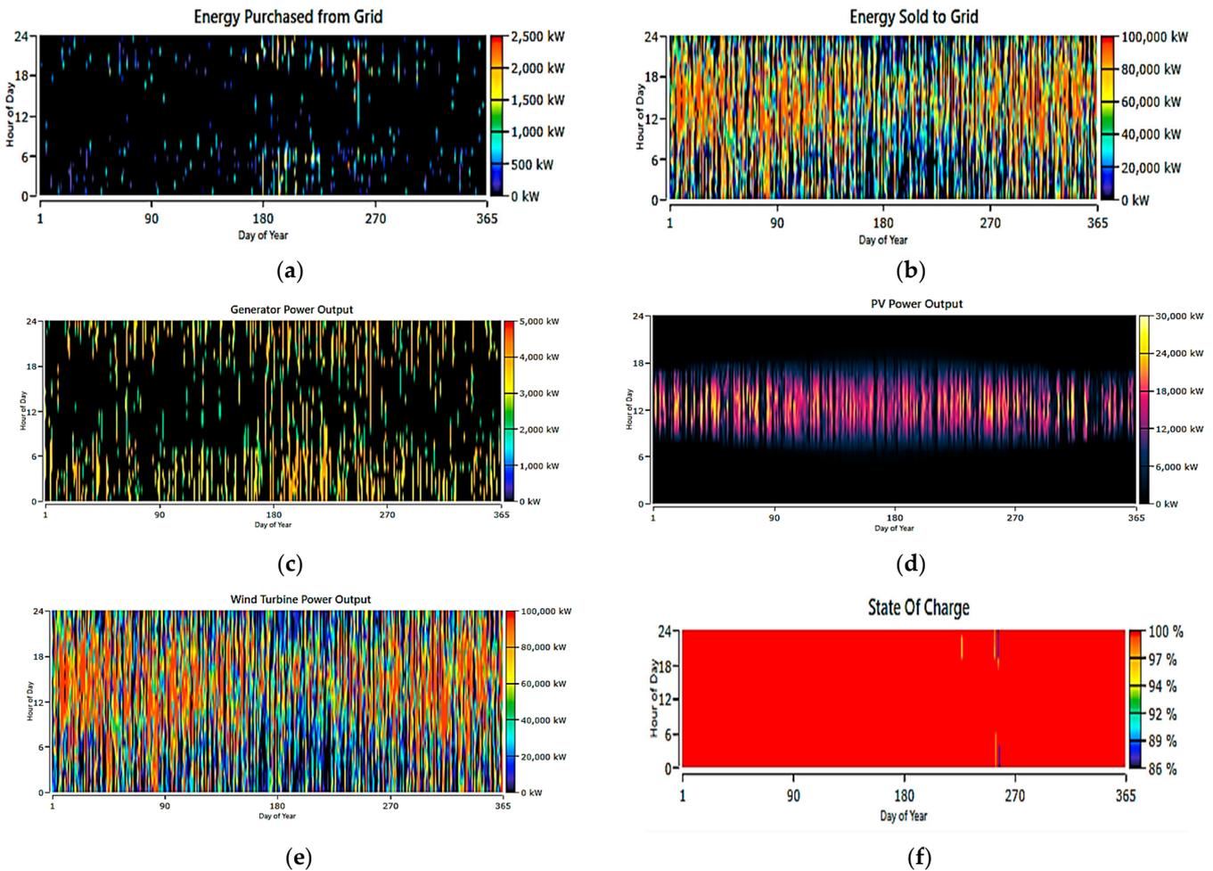
**Figure 20.** System 5: grid, CHP, PV, ESS, and wind (a) energy purchased from grid, (b) energy sold to grid, (c) CHP output power, (d) PV output power, (e) wind power output, and (f) state of charge.
