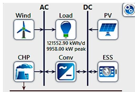
**Figure 21.** System 6: CHP, WT, PV, and ESS design.
