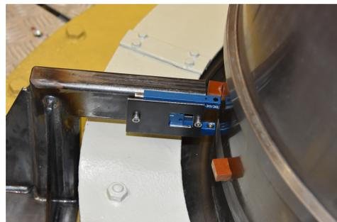
**Figure A13.** Lower sensor installation above the turbine guide bearing.
