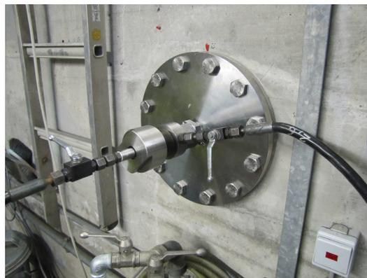
Figure A10. Leakage water—access point and dynamic pressure probe.
