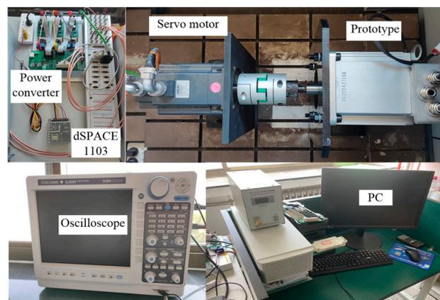
**Figure 15.** Testing platform of the prototype.
