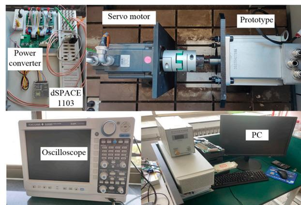
**Figure 15.** Testing platform of the prototype.
