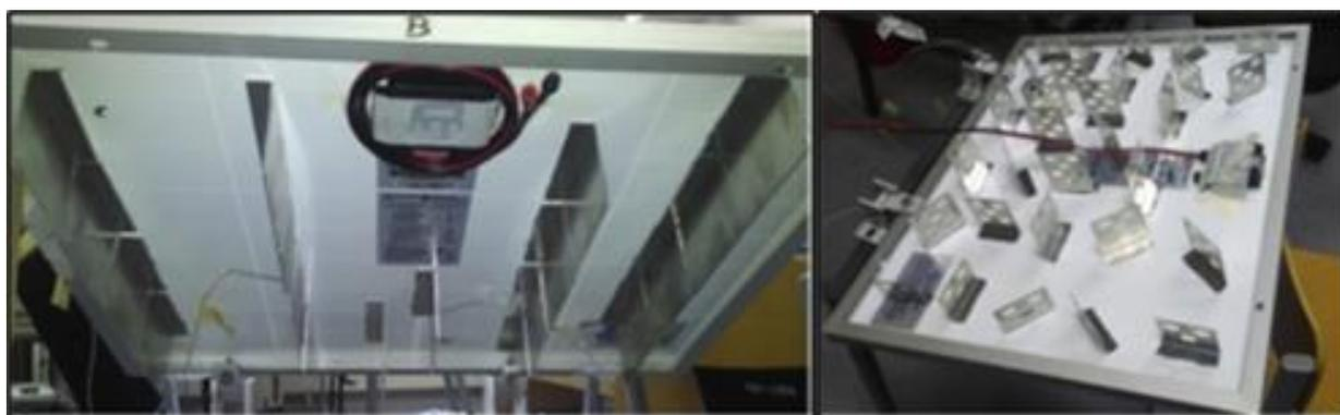
**Figure 1.** Linear and random perforated fins [25].
