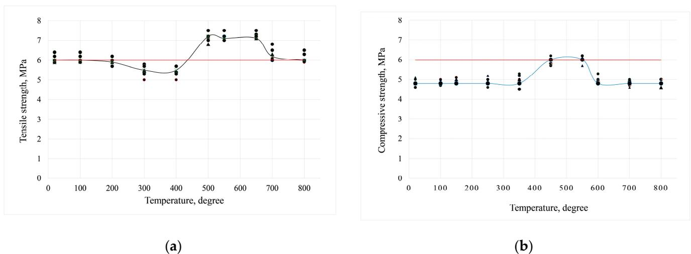
**Figure 6.** Changes in the ultimate tensile strength of chamotte refractories depend on temperature (blue line—obtained dependence; red line—tensile strength at a temperature of 20 degrees). (a)—for new refractories; (b)—for refractories after three fuses.
