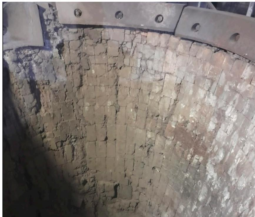
**Figure 1.** The state of the masonry of casting ladle after five fuses.
