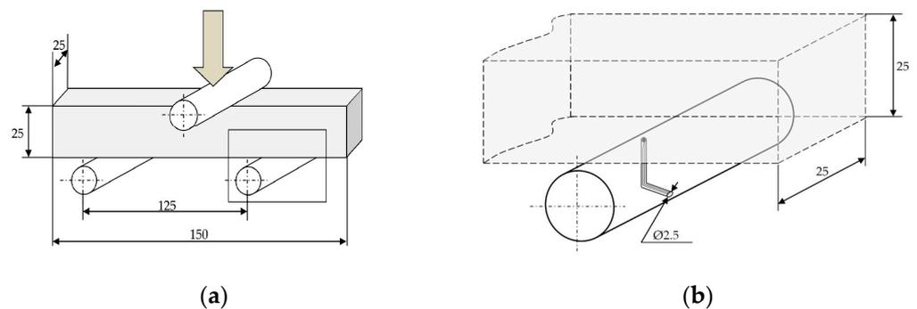
**Figure 3.** Scheme of the method for determining the ultimate tensile strength (a) and the method of installing thermocouples in roller supports (b).
