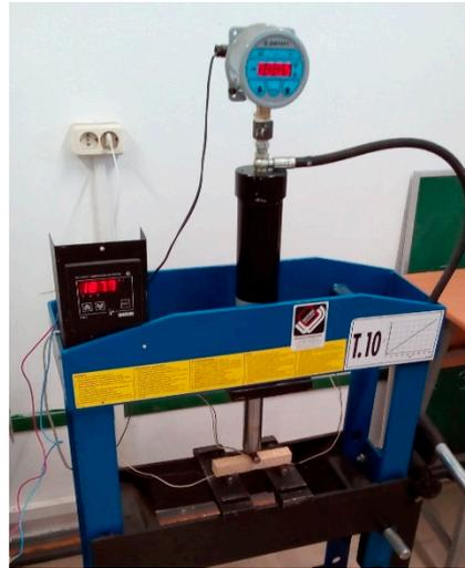
Figure 4. Research setup for determining the ultimate tensile strength.
