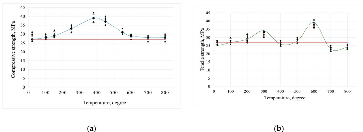
Figure 5. Changes in the ultimate compression strength of chamotte refractories depend on temperature (blue line—obtained dependence; red line—tensile strength at a temperature of 20 degrees). (a)—for new refractories; (b)—for refractories after three fuses.
