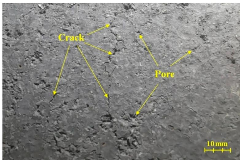
**Figure 2.** Condition of the refractory brick from the working layer of the lining.
