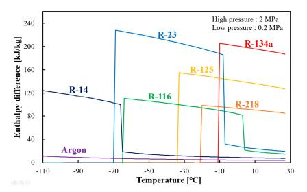
**Figure 3.** Differential enthalpy per unit mass between high and low pressure along the isothermal lines.
