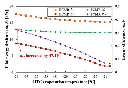
Figure 9. Exergy analysis according to the HTC evaporation temperature.
