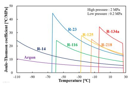
Figure 4. Joule-Thomson coefficient with operating pressure.
