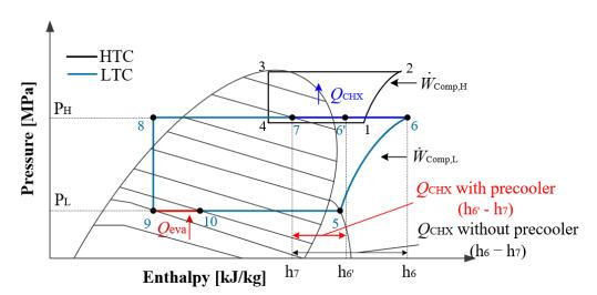
**Figure 2.** P-h diagram of the PCMR J-T cycle.
