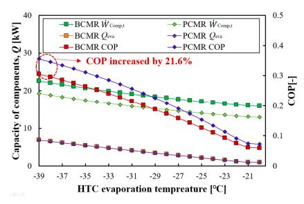
Figure 5. Performance comparison of the system according to HTC evaporation temperature.
