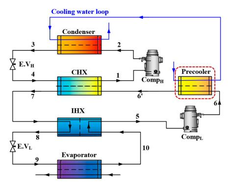
Figure 1. Schematic of the PCMR J-T cycle.
