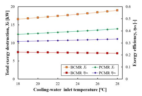
Figure 10. Exergy analysis according to the cooling water temperature.
