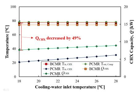
Figure 8. LTC side CHX inlet temperature and capacity variations with cooling water temperature.
