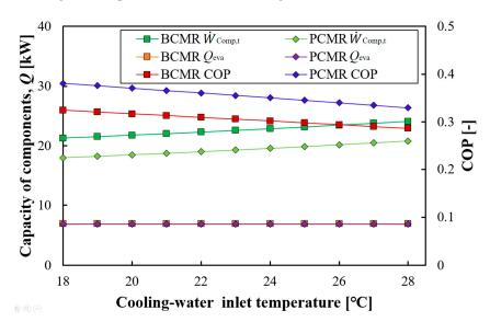
Figure 6. Performance comparison of the system according to cooling water temperature.
