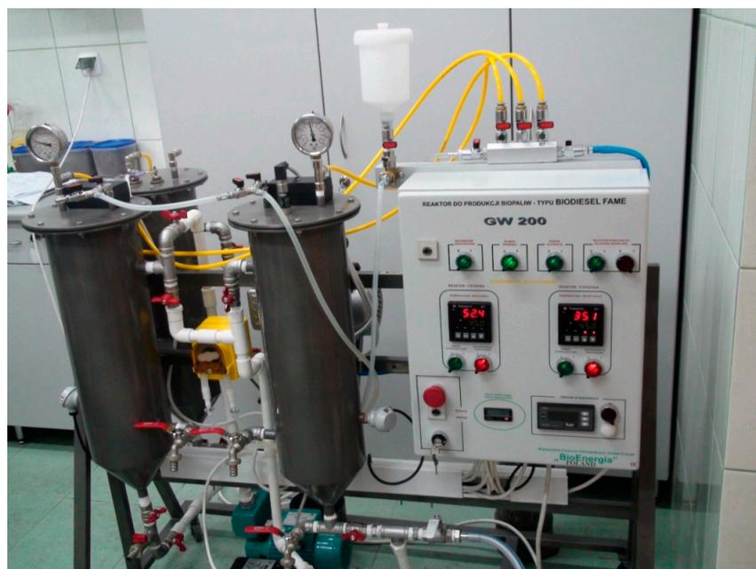
**Figure 1.** GW 200 reactor making vegetable oil esters to fuel diesel engines.
