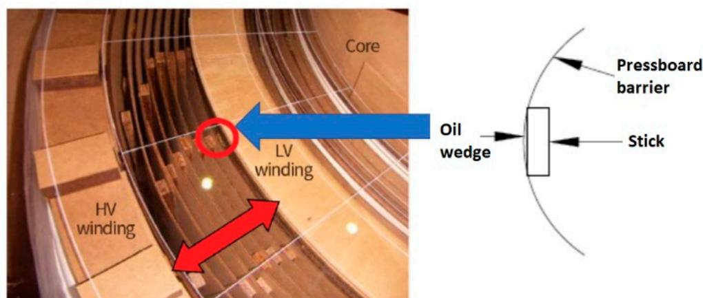
Figure 1. Example of the place of occurrence of an oil wedge in a transformer [14].
