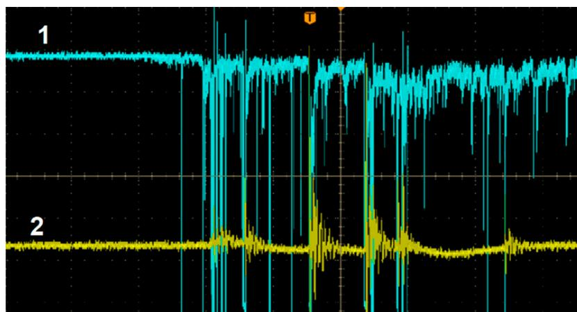
**Figure 4.** Example of oscillogram registered when partial discharge started to develop: 1—light signal from PMT, 2—signal from coupling quadrupole; x-axis represents time ( $t = 4 \mu\text{s}/\text{div.}$ ), y-axis represents voltage in relative units.
