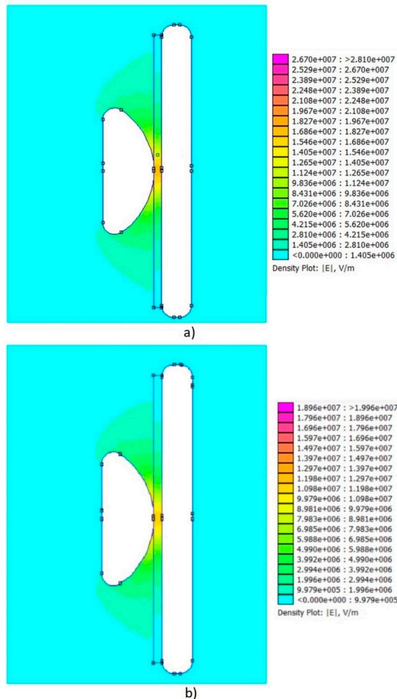
**Figure 7.** Electric field distribution in the model electrode system for the examples of: (a) mineral oil as dielectric liquid, (b) synthetic ester as dielectric liquid.
