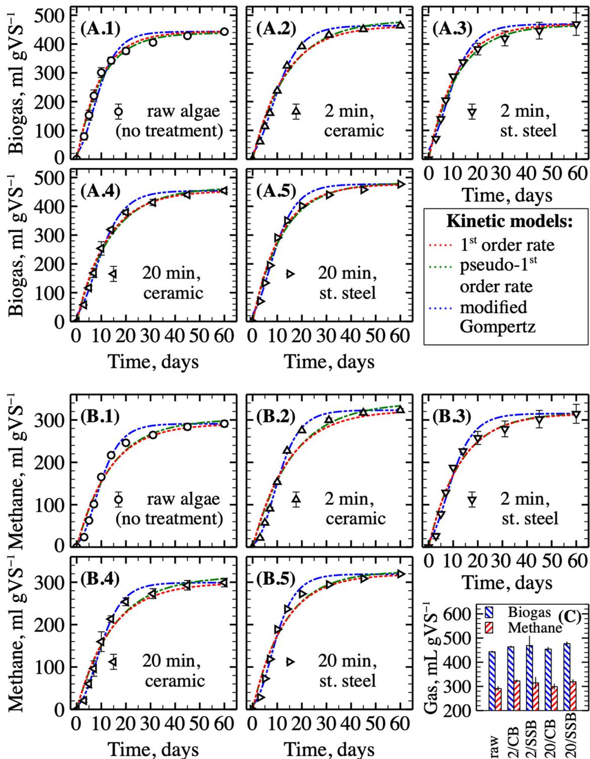
**Figure 2.** Experimental (markers) and model predicted (lines) production of biogas (A.1–A.5) and methane (B.1–B.5) from raw algal–bacteria biomass and biomass milled with either ceramic ball (CB) or stainless steel balls (SSBs) for either 2 or 20 min. Model yields calculated using the 1st-order equation (dotted line), pseudo-1st-order equation (dash-dot line) and modified Gompertz equation (dash-dot-dot line). Ultimate yields for biogas and methane are compared on panel (C).
