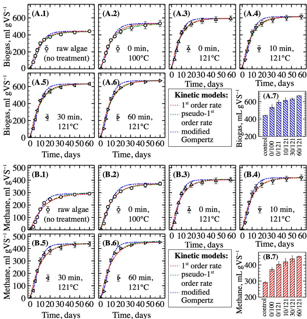
**Figure 4.** Experimental (markers) and model predicted (lines) production of biogas (A.1–A.6) and methane (B.1–B.6) from raw and thermally pretreated algal–bacteria biomass. Model yields calculated using the 1st-order equation (dotted line), pseudo-1st-order equation (dash-dot line) and modified Gompertz equation (dash-dot-dot line). Ultimate yields for biogas and methane are compared on panel (A.7) and (B.7), respectively.
