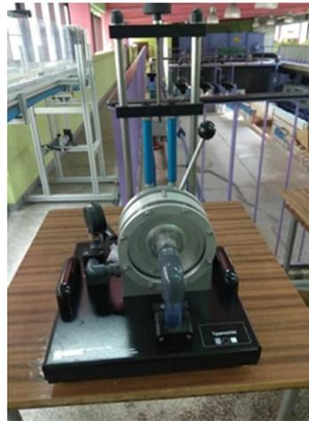
**Figure 1.** Francis turbine GUNT HM 150.20 (GUNT Geraetebau GmbH, Barsbüttel, Germany) used in model tests (K. Mastalerek).
