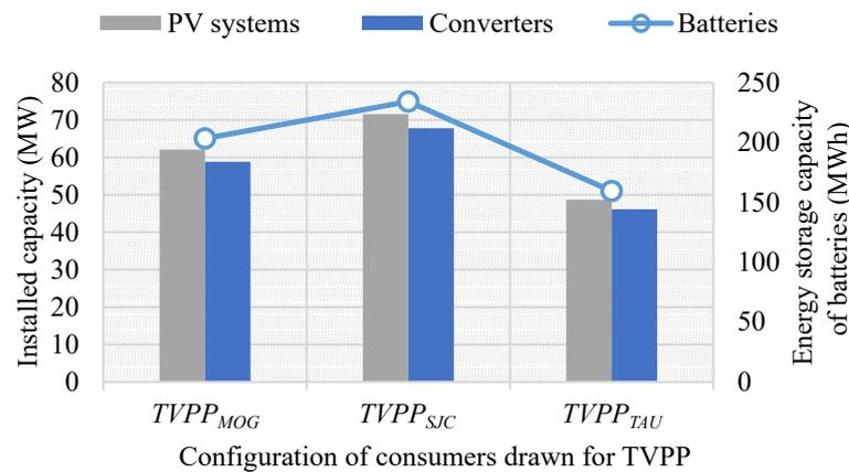
**Figure 6.** Aggregated capacity of DERs of the TVPPs.
