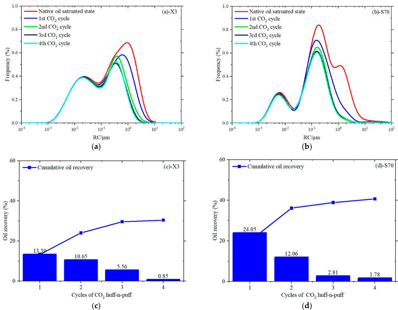
**Figure 3.** The performance of CO<sub>2</sub> huff-n-puff. (a) X3 sample. (b) S70 sample. Oil recovery at different cycles. (c) X3 sample. (d) S70 sample.
