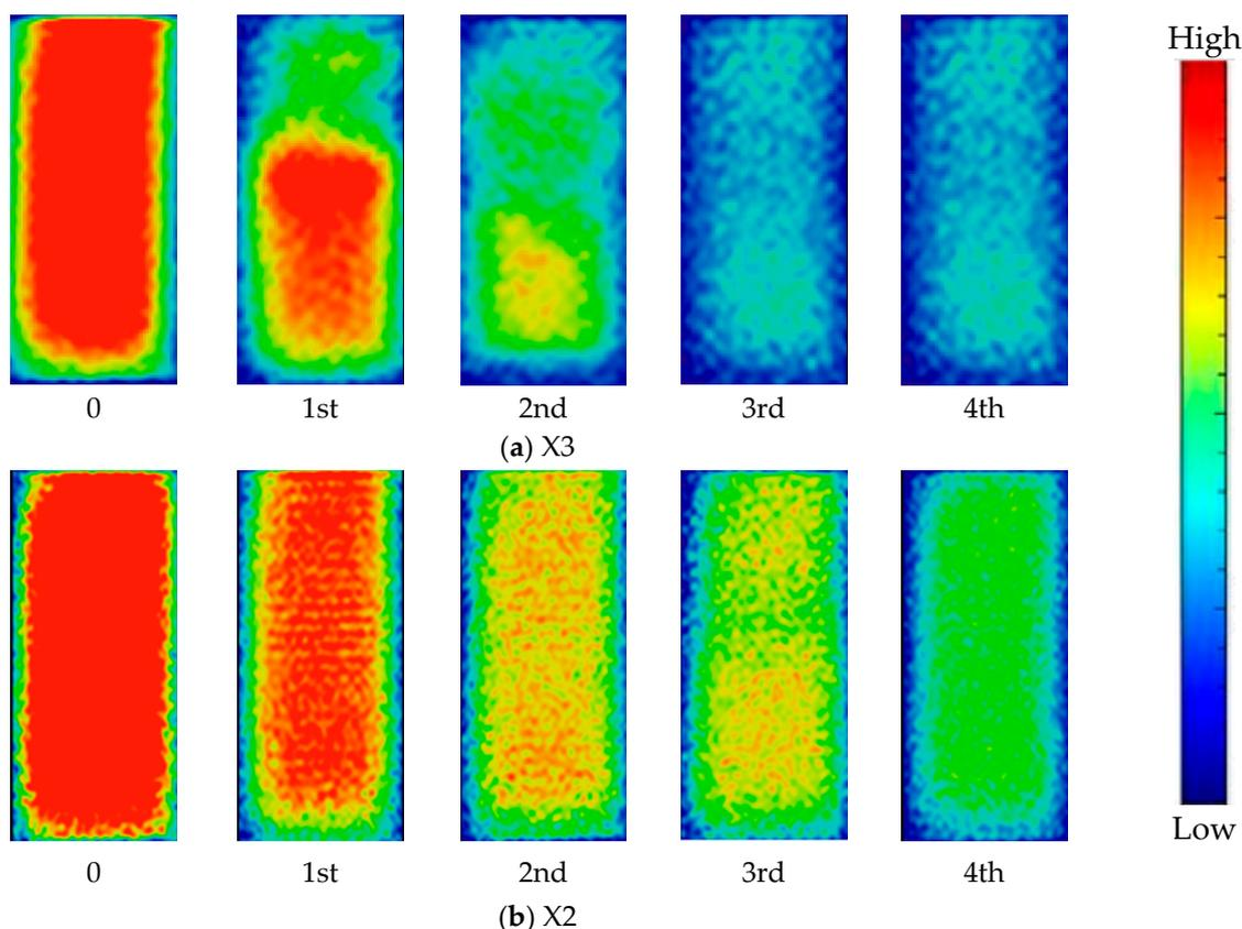
**Figure 6.** (a) The NMR images of oil saturated X3 sample at different CO<sub>2</sub> huff-n-puff cycles. (b) The NMR images of oil saturated X2 sample at different surfactant imbibition cycles.
