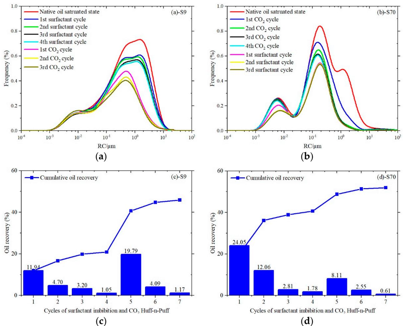
**Figure 5.** The performance of varied injection sequences. (a) S9 sample. (b) S70 sample. The cumulative oil recovery at different cycles. (c) S9 sample. (d) S70 sample.
