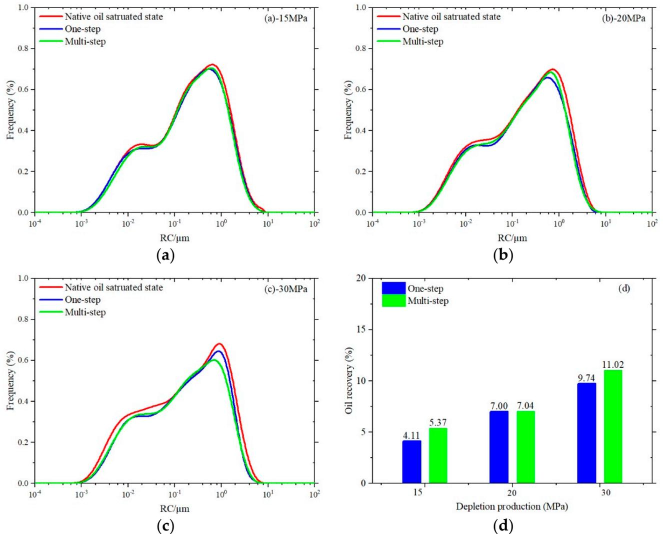
**Figure 2.** The performance of shale oil under depletion production. (a) Comparison of 15 MPa one-step and multi-step depletion production. (b) Comparison of 20 MPa one-step and multi-step depletion production. (c) Comparison of 30 MPa one-step and multi-step depletion production. (d) Comparison of the oil recovery by one-step and multi-step depletion production at different initial pressures.
