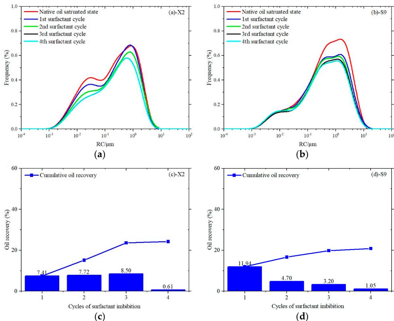
**Figure 4.** The performance of surfactant imbibition. (a) X2 sample. (b) S9 sample. The cumulative oil recovery at different cycles. (c) X2 sample. (d) S9 sample.
