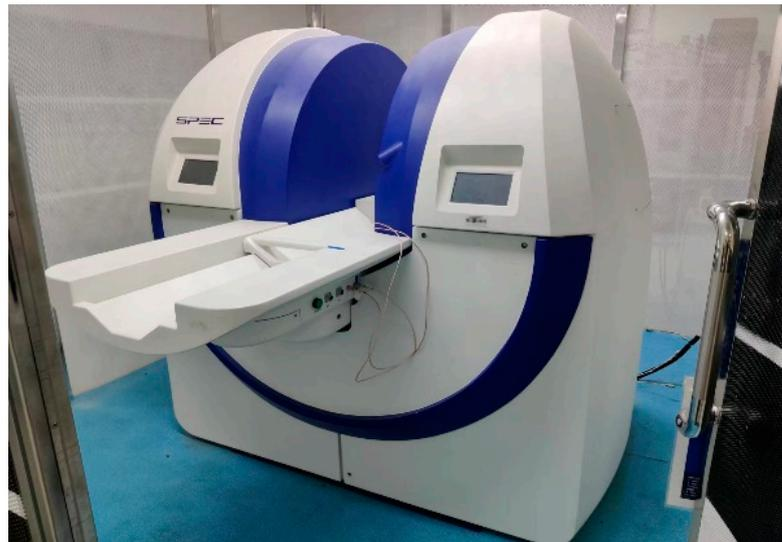
Figure 1. NMR online displacement system.
