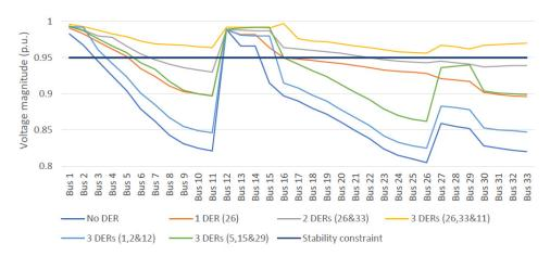
Figure 7. Voltage profile improvement with DER units placement.
