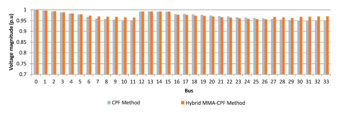
**Figure 13.** Voltage magnitude after DER integration with the CPF method and the proposed hybrid method.
