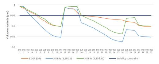
Figure 10. Comparison of voltage profile.
