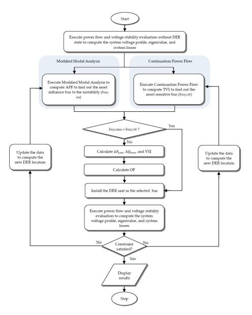
Figure 1. The hybrid MMA-CPF DER allocation approach flowchart.
