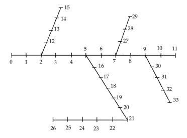
Figure 2. IEEE 34-bus distribution network test system [19].
