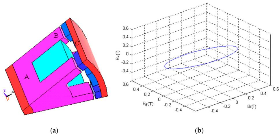
**Figure 4.** Magnetic field finite element analysis: (a) two pole-pitches for numerical analysis, and (b) magnetic flux density locus at Point B when the rotor has rotated by 360 electrical degrees.
