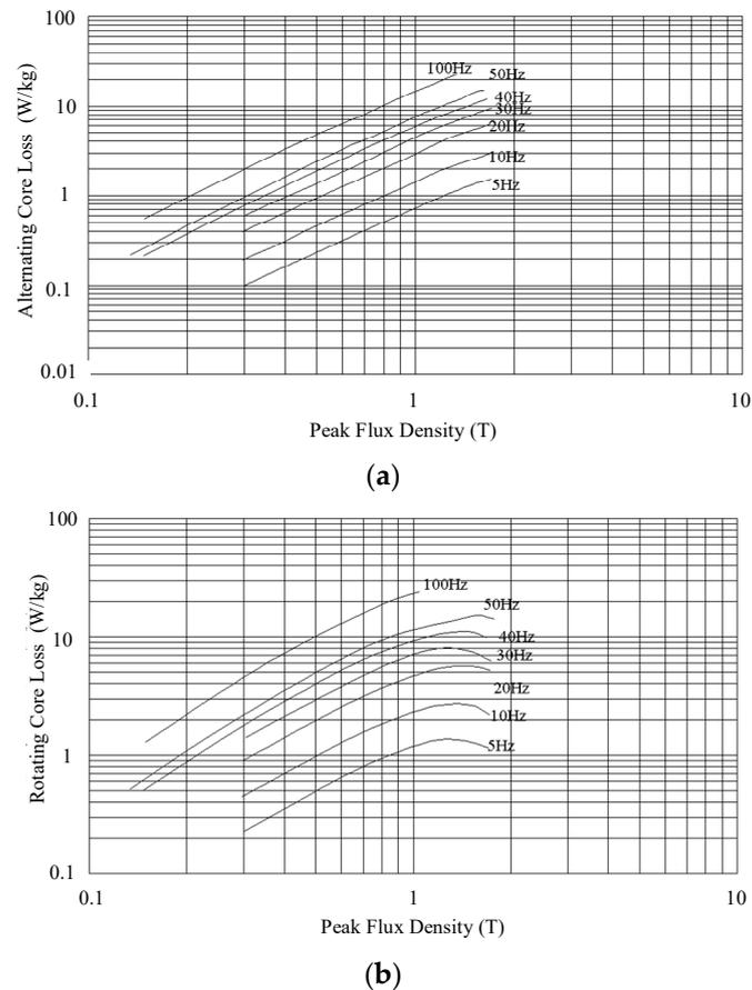
**Figure 6.** Measured core losses of SMC sample: (a) with alternating flux, and (b) with circularly rotating flux [156].
