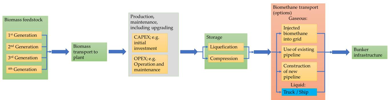
**Figure 7.** Cost constituents of biomethane from source to vessel and port.
