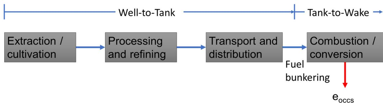
**Figure 6.** WtW supply chain, based on ISWG-GHG 11/2/3 paragraph 3.5 [44], but edited to include possible carbon capture and storage technologies.
