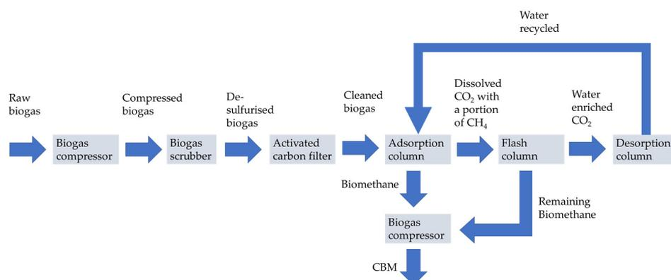
**Figure 11.** WS biogas-to-biomethane upgrading pathway. In addition to WS technology, a scrubber and an activated carbon filter have been added to remove H<sub>2</sub>S and traces of volatile organic compounds (VOCs). The water is recycled for optimal and stable operation. A compressor is preliminarily added for compressed biomethane.
