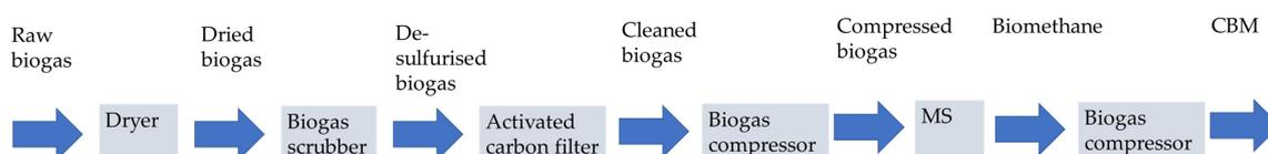
**Figure 10.** MS biogas-to-biomethane upgrading pathway. In addition to MS technology, a scrubber and a drier have been added to remove moisture and H<sub>2</sub>S. The activated carbon filter has also been added to remove traces of H<sub>2</sub>S and volatile organic compounds (VOCs). A compressor is preliminarily added for compressed biomethane.
