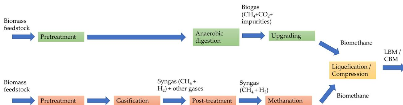
**Figure 1.** Conversion routes to produce liquefied/compressed biomethane.
