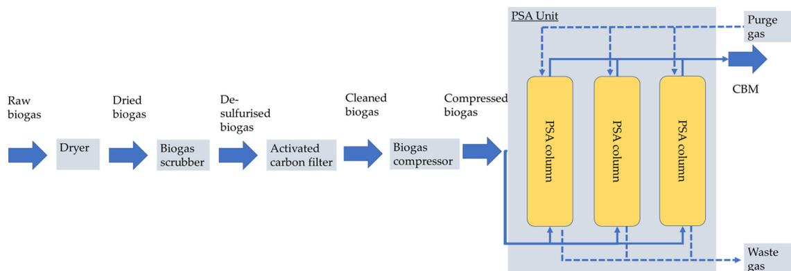
**Figure 13.** PSA biogas-to-biomethane upgrading pathway. In addition to PSA technology, a dryer, a scrubber, and an activated carbon filter have been added to remove moisture,  $H_2S$ , and traces of volatile organic compounds (VOCs). The PSA columns are in connected in series and form the PSA unit.
