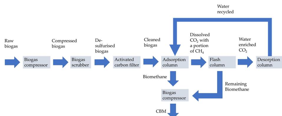
**Figure 11.** WS biogas-to-biomethane upgrading pathway. In addition to WS technology, a scrubber and an activated carbon filter have been added to remove H<sub>2</sub>S and traces of volatile organic compounds (VOCs). The water is recycled for optimal and stable operation. A compressor is preliminarily added for compressed biomethane.
