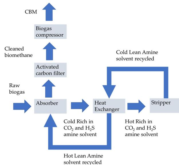
**Figure 12.** CA biogas-to-biomethane upgrading pathway. In addition to CA technology, a scrubber and an activated carbon filter have been added to remove  $H_2S$  and traces of volatile organic compounds (VOCs). The amine solvent is recycled into the absorber as it: a. utilises the heat from the heat exchanger, and b.  $CO_2$  is removed by the stripper. A compressor is preliminarily added for compressed biomethane.
