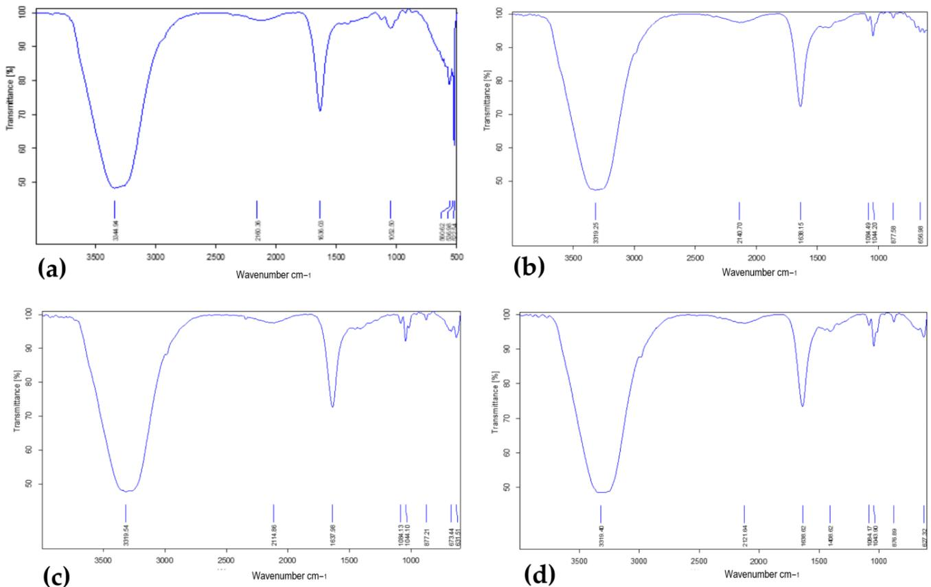
Figure 4. FTIR spectra of (a) Onion extract. (b) Bioethanol from *S. cerevisiae*. (c) Bioethanol from *P. pastoris*. (d) Bioethanol from Co-culture strain.
