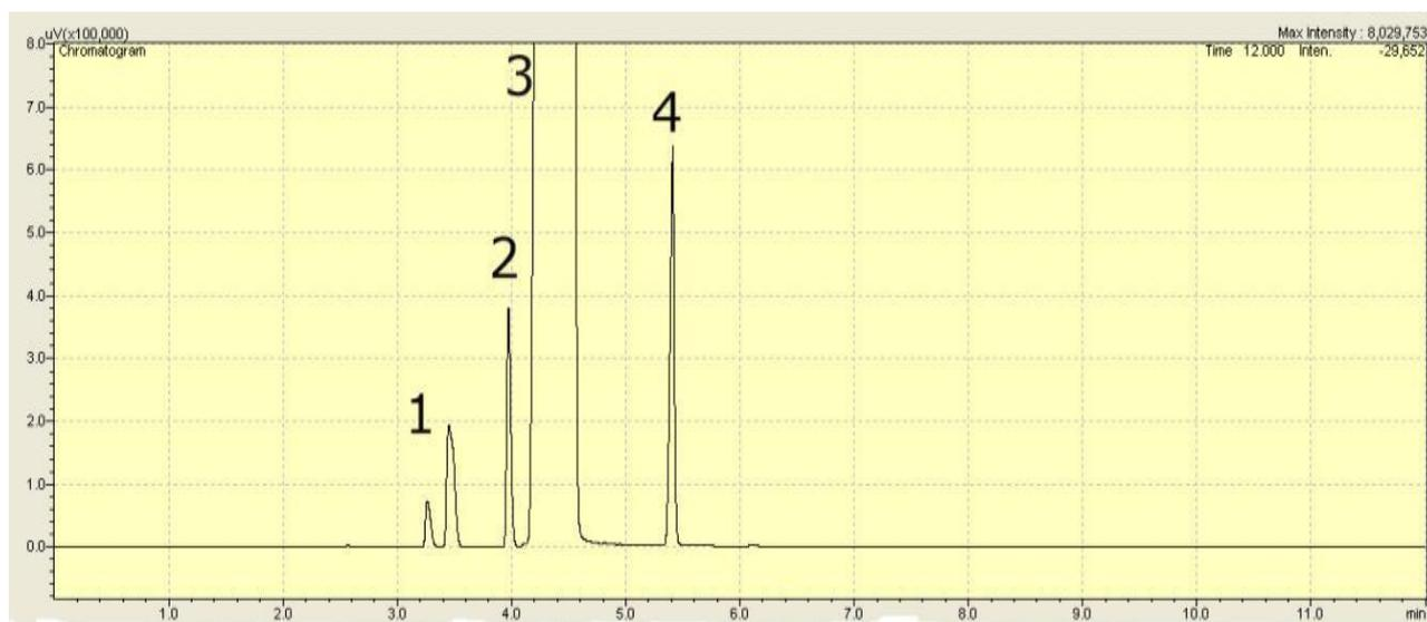
**Figure 5.** A sample chromatogram of GC-FID analysis with peaks; (1). Bioethanol. (2). Acetonitrile. (3). 1-propanol. (4). Butanol.
