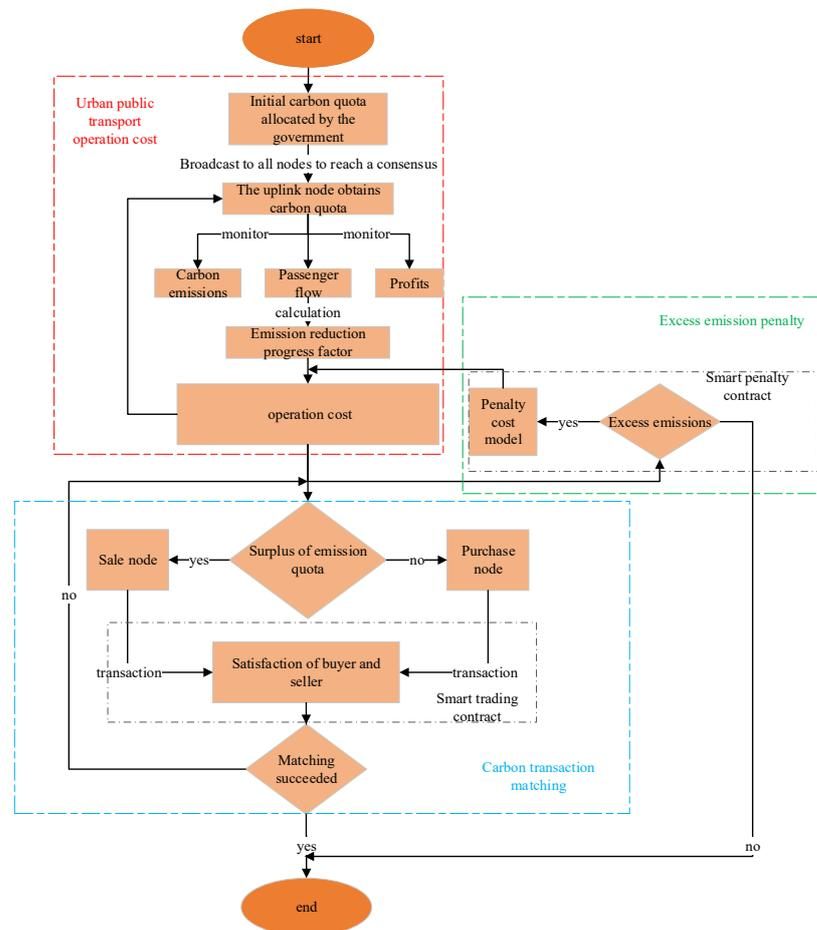
Figure 2. Flow chart of urban public transport carbon-trading system based on blockchain technology.
