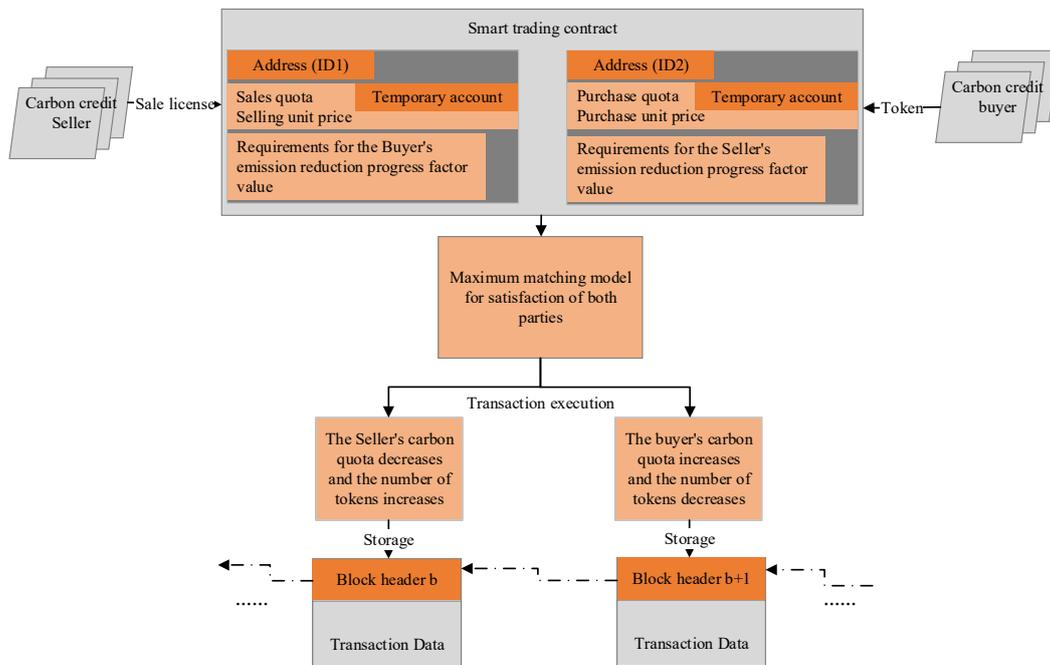
**Figure 3.** Matching model of urban public transport carbon quota transaction based on blockchain technology.
