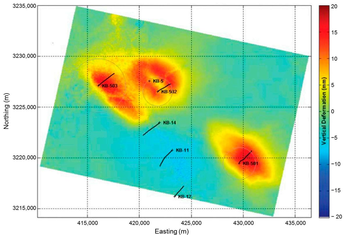
**Figure 6.** Surface deformation observed in CO<sub>2</sub> injection and production wells at the Krechba site (cited in Mathieson A et al., 2010 [38]).
