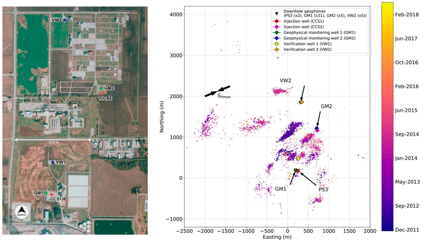
**Figure 7.** IBDP project site monitoring system and event distribution (cited in Bauer et al., 2019 [50] and D E Dando et al., 2021 [51]).
