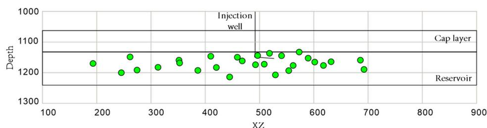
**Figure 12.** Location of microseismic events (green dots are microseismic events).
