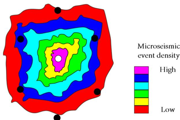
**Figure 8.** A schematic diagram of microseismic monitoring results in the Jilin work area in China (modified according to Ren B et al., 2016 [63]; white dots are injection wells and black dots are production wells).
