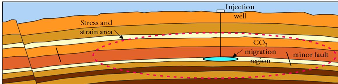
**Figure 2.** Schematic diagram of reservoir changes after CO<sub>2</sub> injection into the reservoir (modified from Rutqvist J, 2012 [9]).
