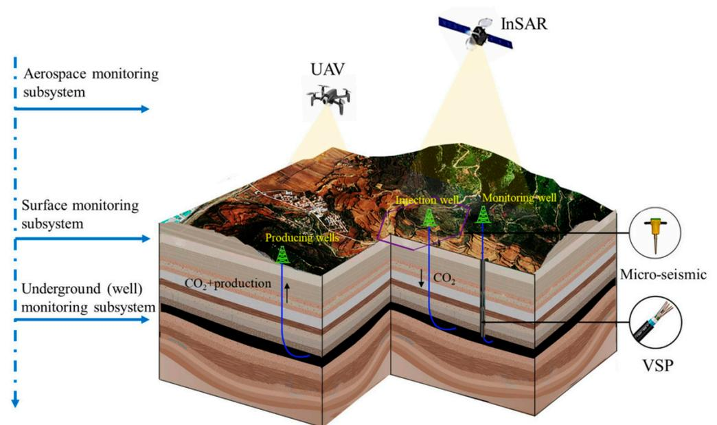
**Figure 9.** Schematic diagram of the monitoring system of the Shanxi project (cited in Tian Z et al., 2022 [64]).
