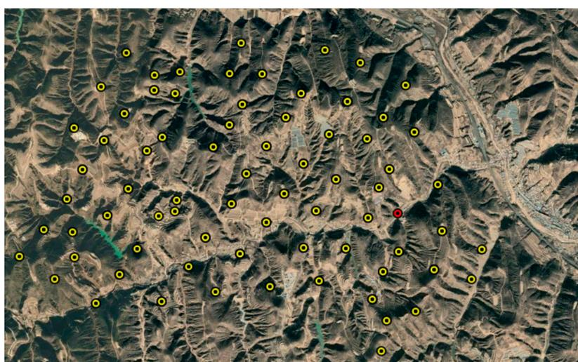
**Figure 11.** Combined well and ground observation system (red dot in the figure is the position of instruments in the well, and yellow dots are the positions of instruments on the ground).
