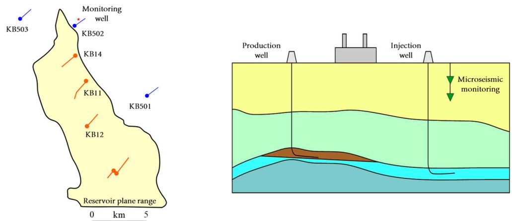
**Figure 5.** Schematic of the Krechba field showing the location of injection and production wells (modified from Stork A L et al., 2015 [36]); the figure shows injection wells in blue and production wells in orange, and star symbol is the monitoring well).
