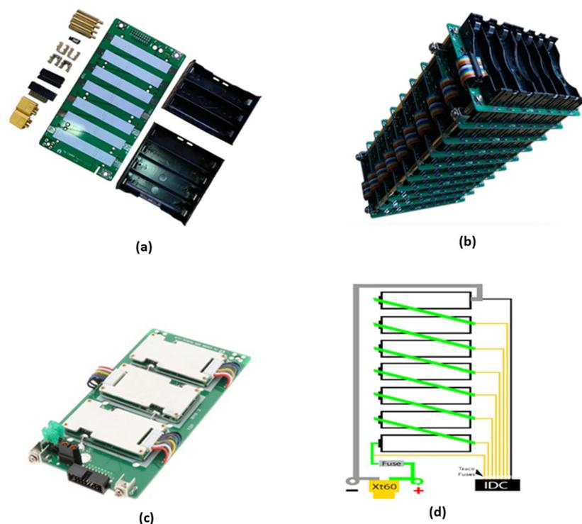
**Figure 12.** Open-source, Do-it-yourself modular battery storage kit: (a) exploded view; (b) assembled and stacked; (c) battery management module; (d) simplified circuit representation of the battery module [128].
