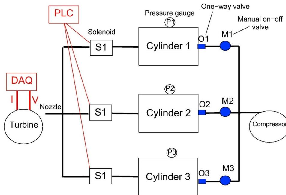
**Figure 14.** Main components of the modular low-pressure micro-CAES [146].
