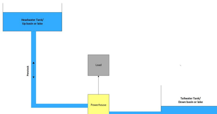
**Figure 6.** Working principle of pumped hydroelectric storage stations.
