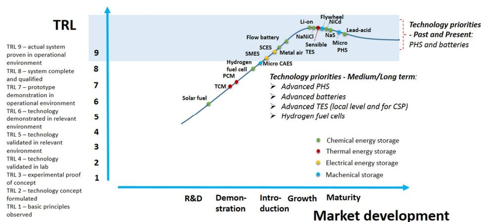
**Figure 11.** Overview of the maturity of energy storage technologies (Thermo-Chemical Materials (TCMs), phase change materials (PCMs), superconducting magnetic energy storage (SMES), super capacitor energy storage (SCES), sodium nickel chloride (NaNiCl) batteries, thermal energy storage (TES), nickel cadmium (NiCd) batteries, sodium sulphur (NaS) batteries, and pumped hydro storage (PHS)) as of 2017 with technology readiness level (TRL) on the y-axis and market development on the x-axis [120].
