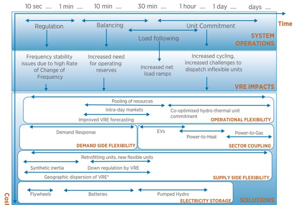
**Figure 5.** Flexibility solutions relevant to intermittent renewable production [52].
