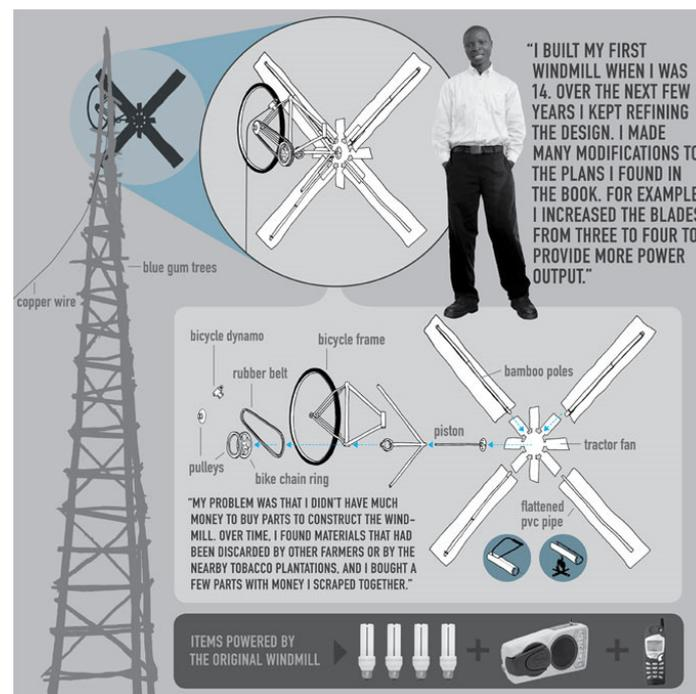
**Figure 3.** William Kamkwamba's windmill design and components [24].
