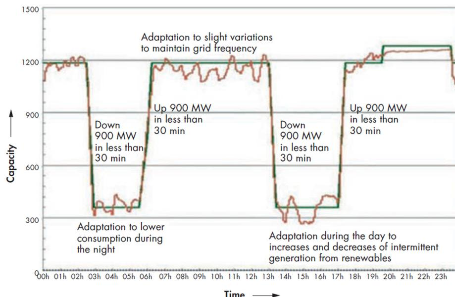
**Figure 8.** Power generated by a 1300 MW nuclear reactor over 24 h in response to grid variations.
