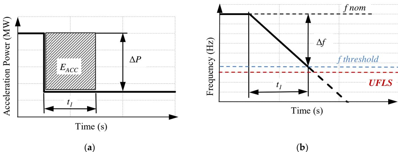
**Figure 1.** (a) Fixed acceleration power; (b) linear frequency deviation.
