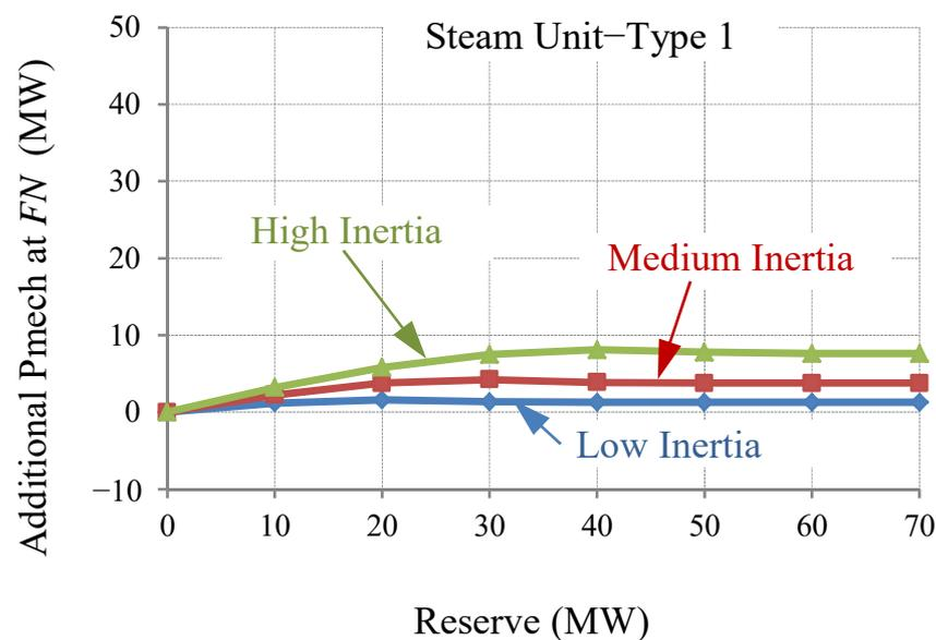
**Figure 4.** Additional mechanical power of Steam Unit—Type 1 as response for 350 MW trip, in 3 inertia conditions.
