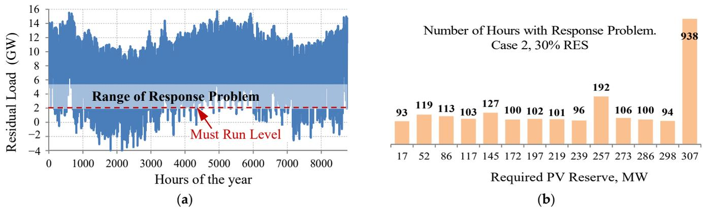
**Figure 12.** (a) Residual Load through the year 2030; (b) distribution of necessary PV reserve in the Range of the Response Problem, Case 2.
