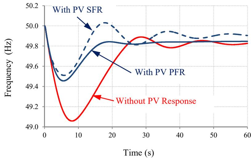
**Figure 10.** System frequency response to 350 MW generator trip, at minimum Residual Load point of the year 2030, Case 1.
