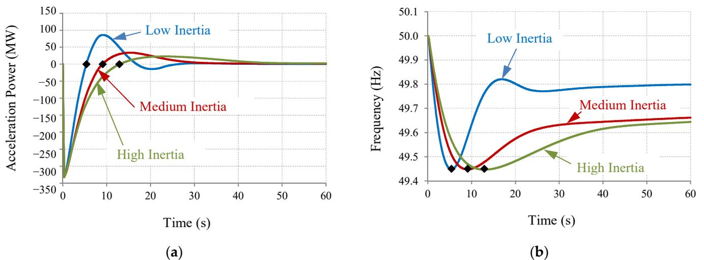
Figure 3. (a) Acceleration power; (b) frequency; in the Israeli power system after 350 MW generation trip, different inertia conditions.
