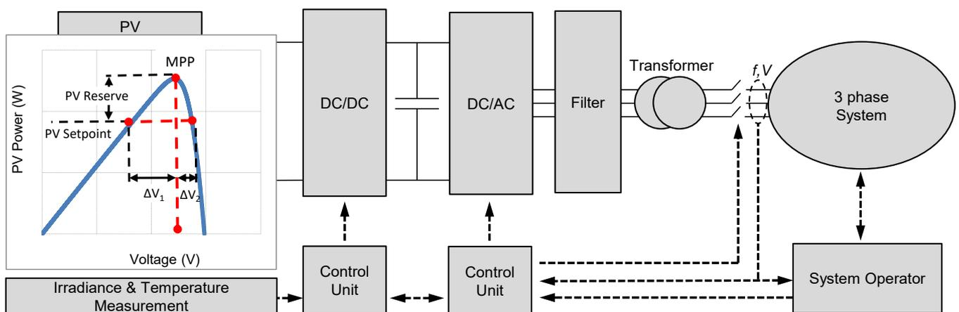
Figure 7. A principal scheme of PV facility with frequency-power control.
