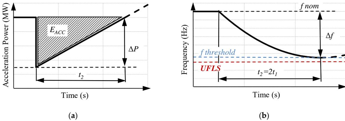
Figure 2. (a) Linear change in acceleration power; (b) quadratic frequency deviation.
