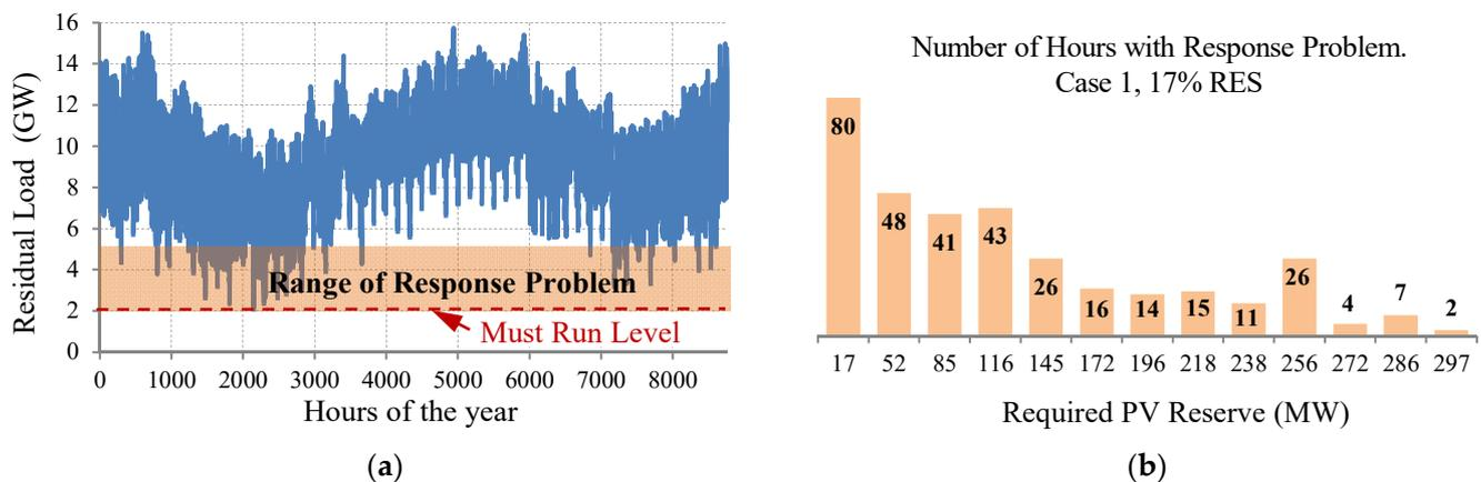
**Figure 11.** (a) Residual Load through the year 2030; (b) distribution of necessary PV Reserve in the Range of the Response Problem, Case 1.
