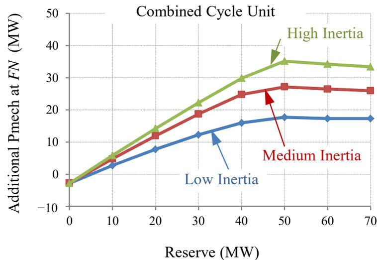
**Figure 6.** Additional mechanical power of Combined Cycle Unit as response for 350 MW trip, in 3 inertia conditions.
