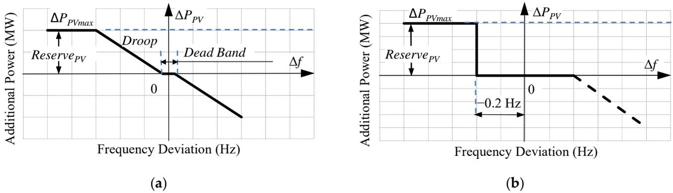
Figure 8. Two types of PV plant frequency response: (a) PFR; (b) SFR.
