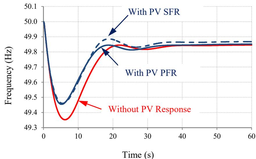
**Figure 9.** System frequency response to 350 MW generator trip, at minimum residual load point of the year 2021, Case 1.
