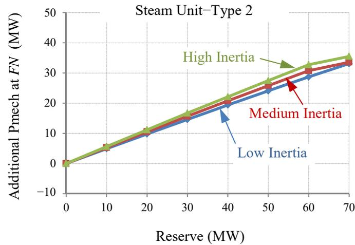
**Figure 5.** Additional mechanical power of Steam Unit—Type 2 as response for 350 MW trip, in 3 inertia conditions.
