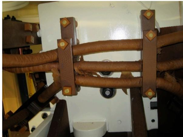
**Figure 1.** Damaged insulation during short circuit test.
