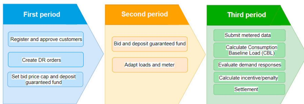
**Figure 3.** The demand response bidding mechanism.
