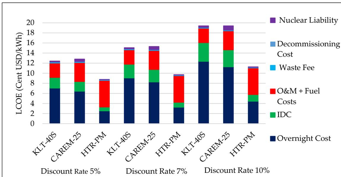
Figure 8. Graph of the distribution of cost components of CAREM-25, KLT-40S, and HTR-PM LCOE with various discount rates.
