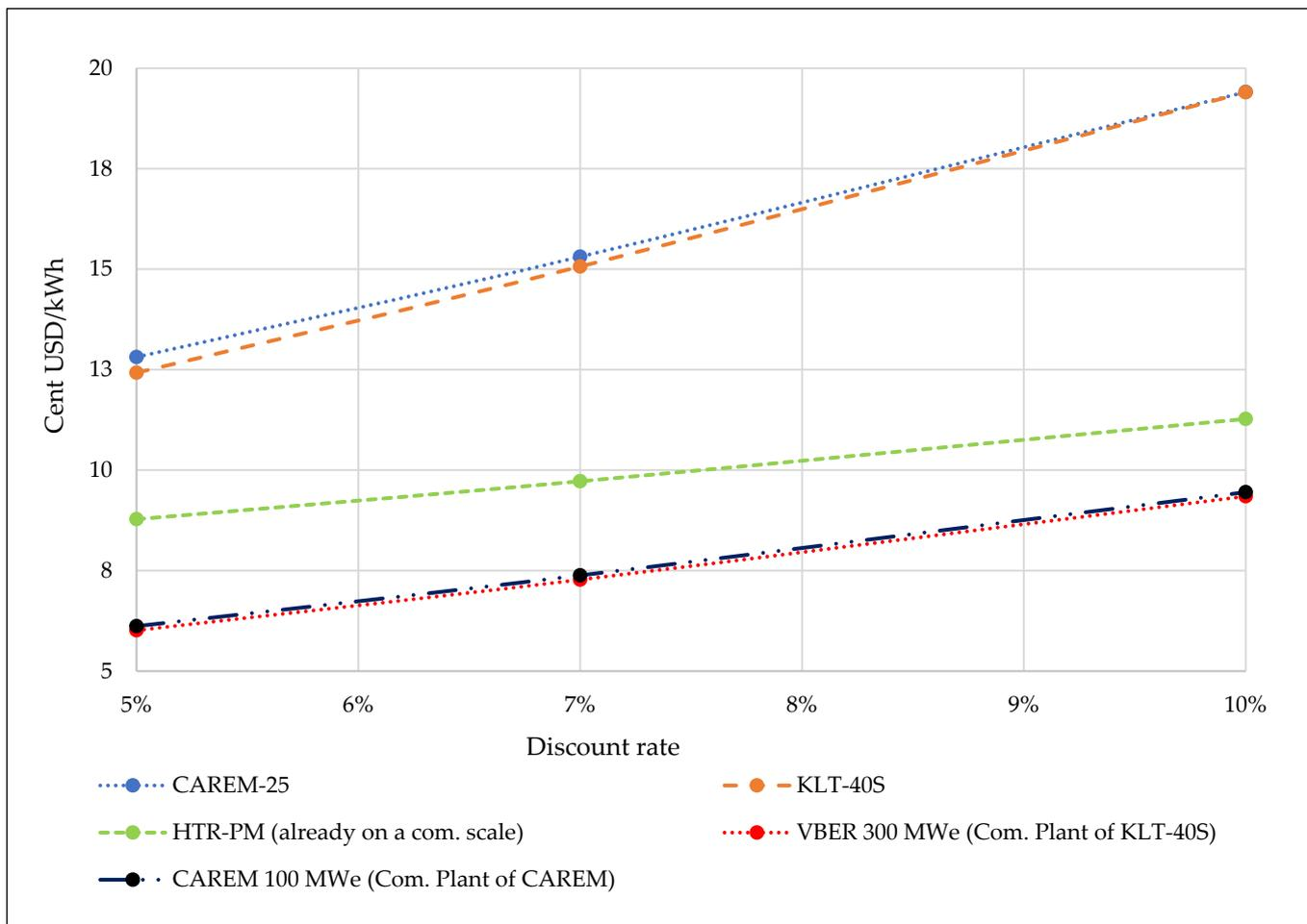
Figure 7. Graph of CAREM-25, KLT-40S, and HTR-PM LCOEs with various discount rates.
