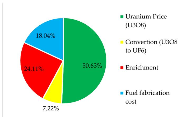
Figure 6. Cost component for 1 kg of uranium as  $\text{UO}_2$  fuel [74].
