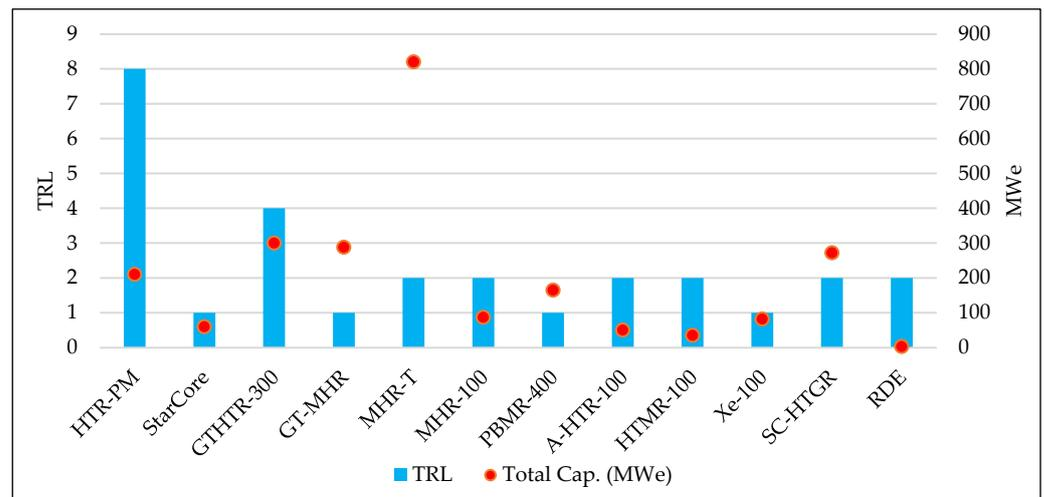
Figure 4. Technology readiness level of high-temperature reactors (HTR) [55,65,68,69].
