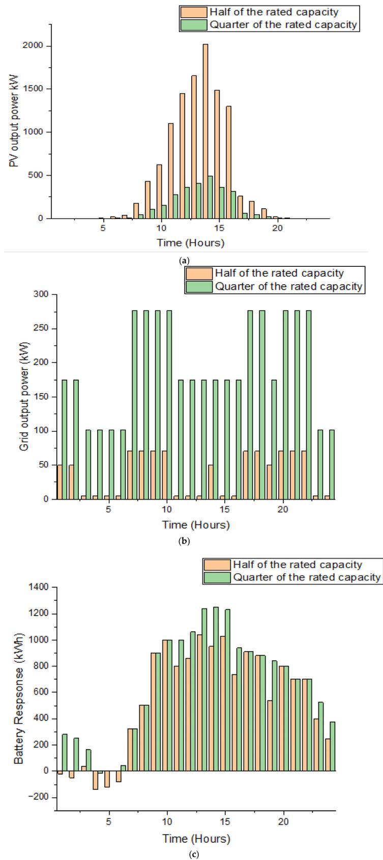
**Figure 10.** (a) P.V. system output power response for P.V. system variation of rated power. (b) Grid output power for P.V. system variation of rated power. (c) Battery storage response for P.V. system variation of rated power.
