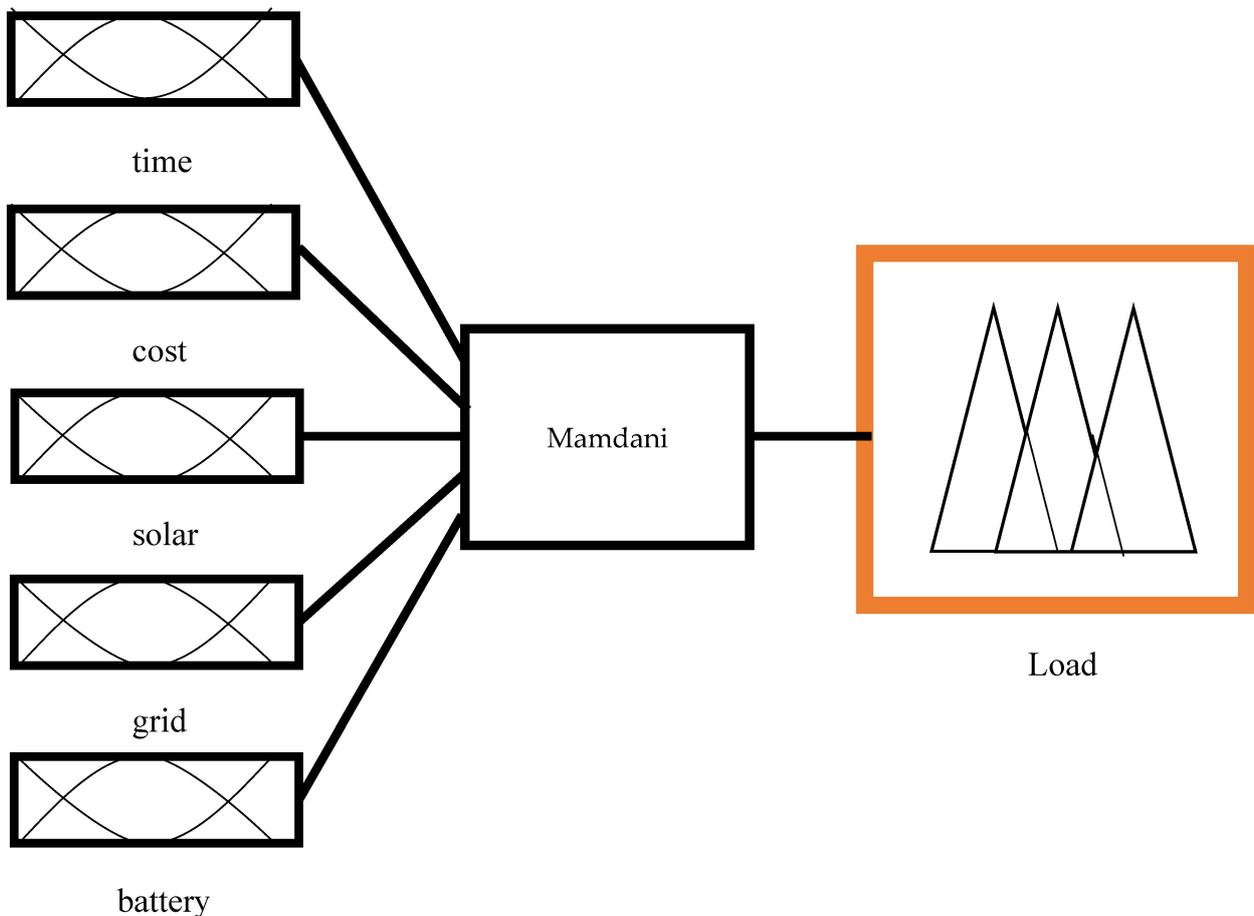
Figure 5. The block diagram of the proposed fuzzy logic controller.
