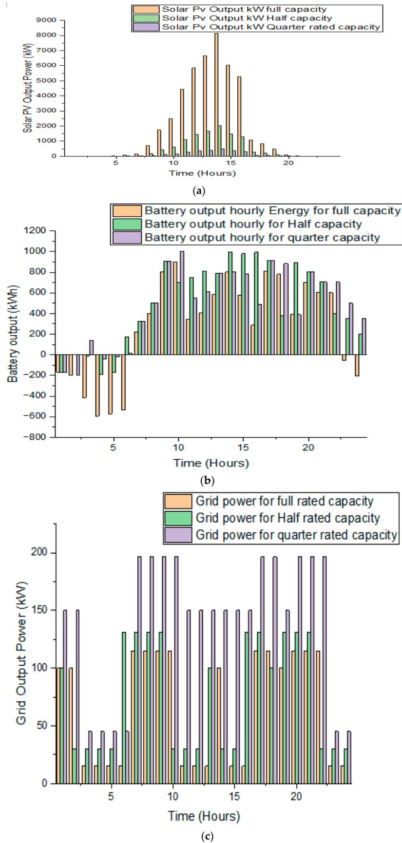
**Figure 6.** (a) Output power of P.V. for full rated power variations. (b) Output variations of battery storage for full rated power. (c) Output power of Grid for full rated power variations.
