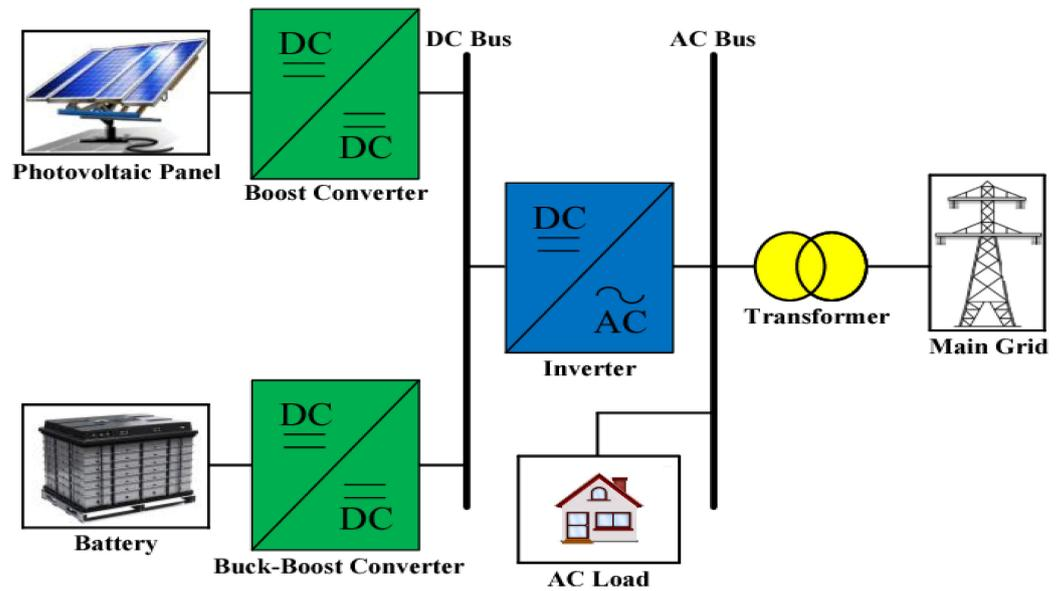
Figure 2. Proposed hybrid Microgrid.
