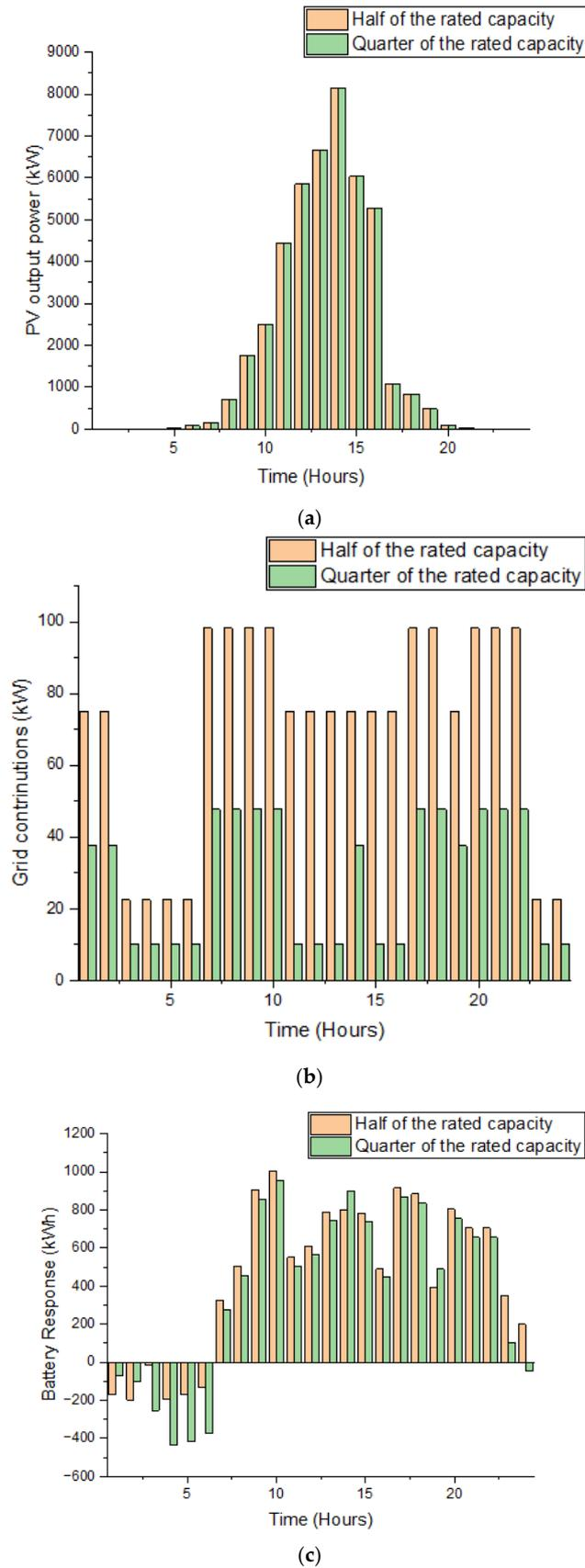
**Figure 12.** (a) P.V. system output power for grid rated power variation. (b) Grid output power for grid rated power variation. (c) Battery storage response for grid rated power variation.
