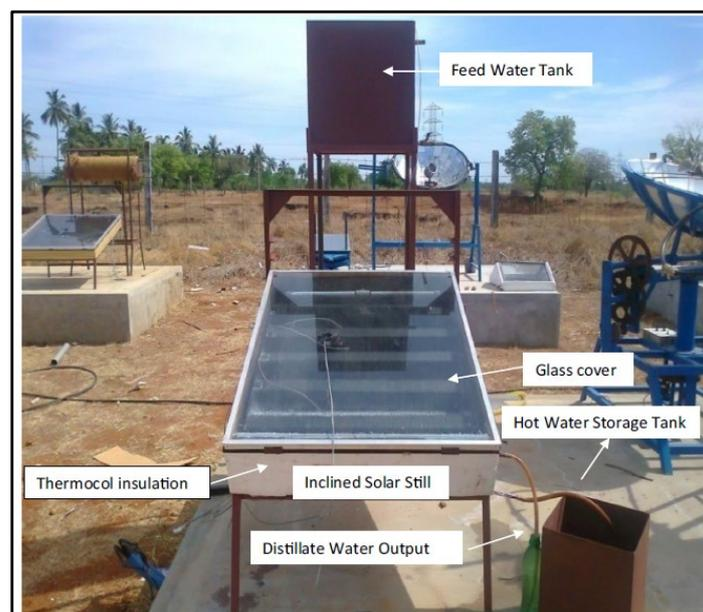
**Figure 11.** Photographic view of the inclined solar still and the wick material [17].
