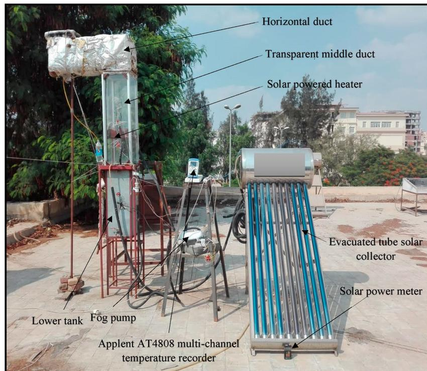
Figure 29. Photograph of the solar-powered fog desalination system [60].
