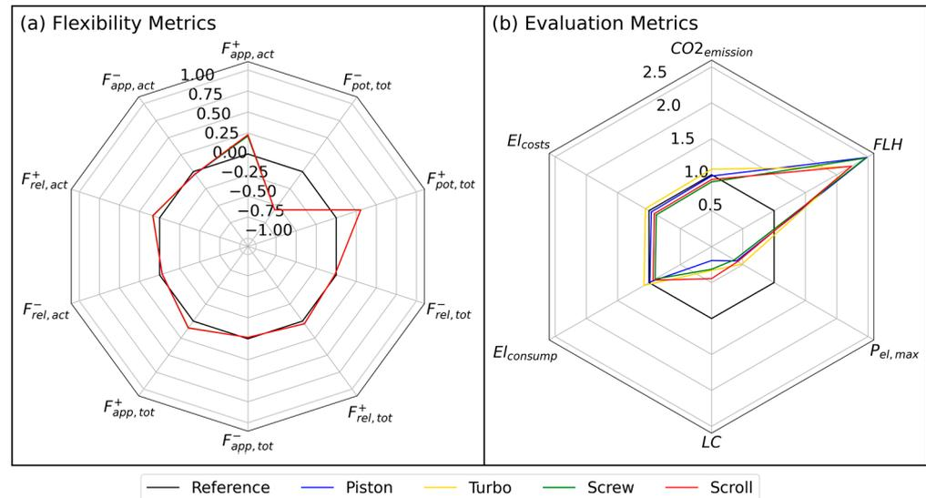
**Figure 8.** (a) Flexibility metrics and (b) evaluation metrics based on the optimized operation of the cold warehouse for the goal “minimization of maximum used electric power”.
