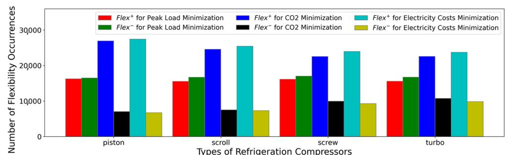
**Figure 5.** Frequency of occurrences of positive and negative flexibility in the optimized operation.
