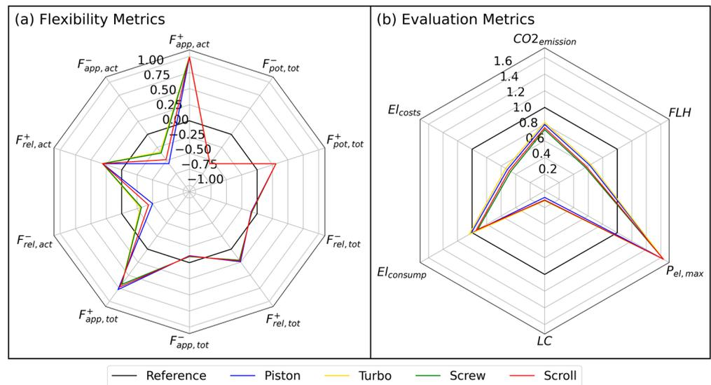
**Figure 6.** (a) Flexibility metrics and (b) evaluation metrics based on the optimized operation of the cold warehouse for the goal “minimization of electricity costs”.
