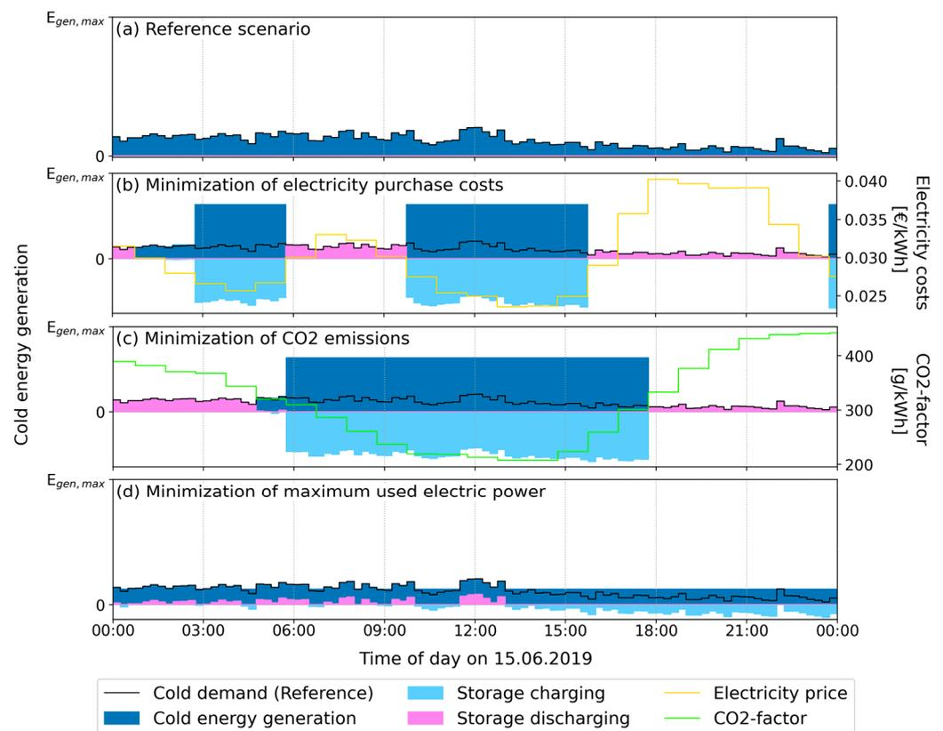
**Figure 3.** Optimized operation of the cold warehouse for (a) reference scenario, (b) minimization of electricity costs, (c) minimization of CO<sub>2</sub> emissions, and (d) minimization of maximum used electric power on 15 June 2019.
