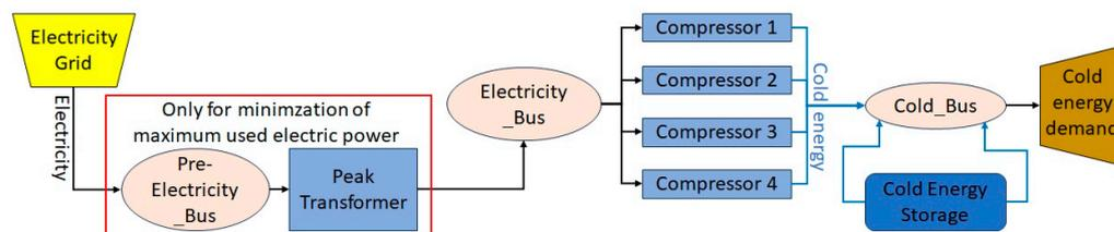
**Figure 1.** Schematic view of the cold warehouse model developed via oemof.
