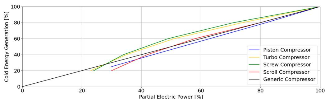
**Figure 2.** Partial load behavior of different types of refrigeration compressors: piston [48], turbo and screw compressors [47], scroll compressor [49], and a generic linear compressor.
