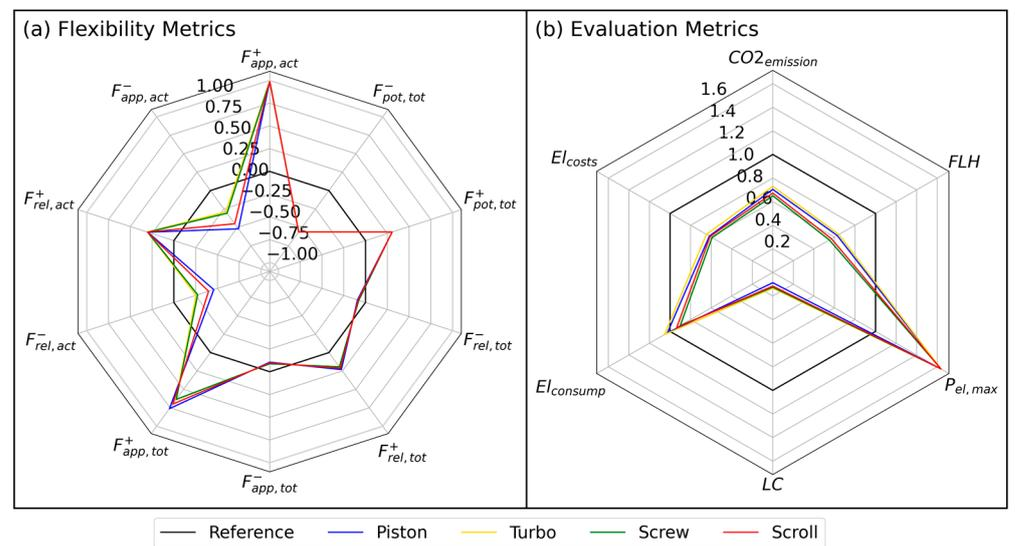
**Figure 7.** (a) Flexibility metrics and (b) evaluation metrics based on the optimized operation of the cold warehouse for the goal “minimization of CO<sub>2</sub> emissions”.
