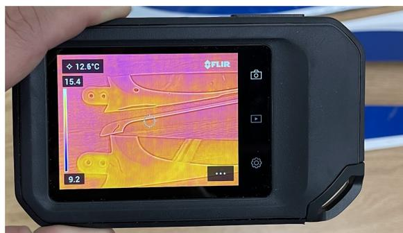
**Figure 8.** FLIR C5 camera, equipped with MSX technology.
