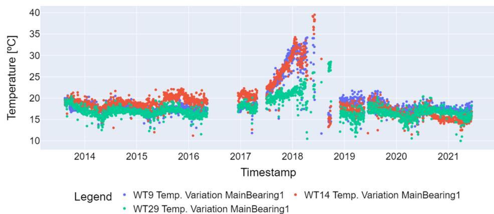
**Figure 5.** Temperature variation for the main bearing after outlier removal (WT9, WT14, and WT29).
