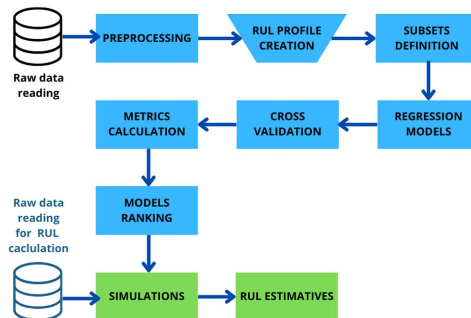
Figure 2. RUL estimation using regression machine learning models.
