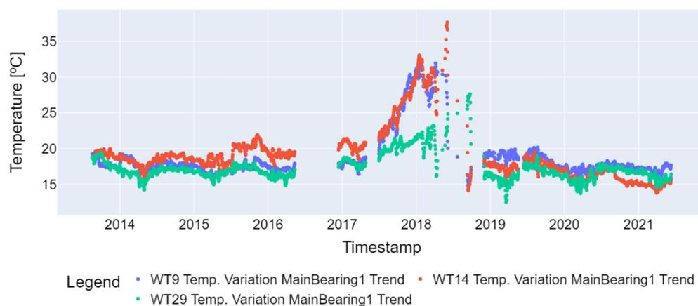
**Figure 6.** Temperature variation for the main bearing after seasonal decomposition (WT9, WT14, and WT29).
