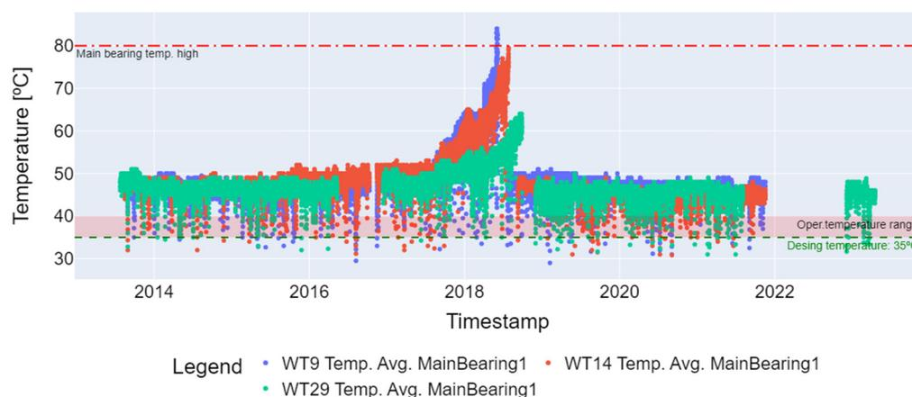
Figure 4. Main bearing average temperature series with outliers (WT9, WT14, and WT29).
