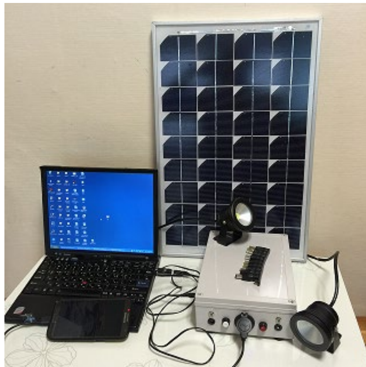
Figure 9. Typical 12 V/14.4 Ah Li-ion SHS.
