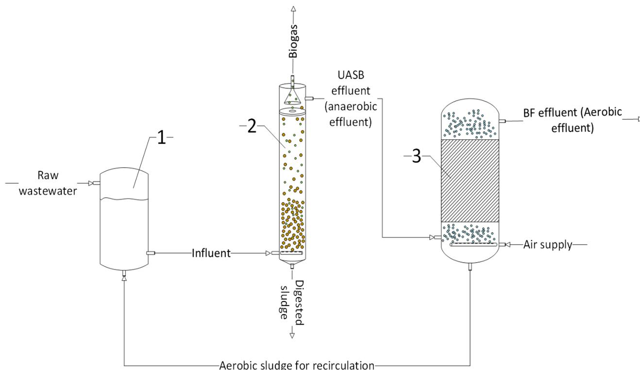
**Figure 9.** A diagram of the UASB-BF system: (1) a storage tank for raw wastewater, (2) a UASB reactor, and (3) a BF; based on [115].
