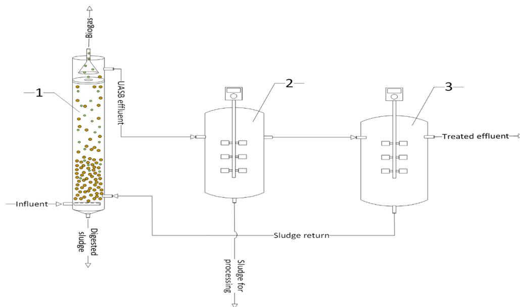
**Figure 7.** A diagram of the UASB–SBR system: (1) a UASB reactor, (2) a UASB effluent storage tank, and (3) an SBR; based on [18].
