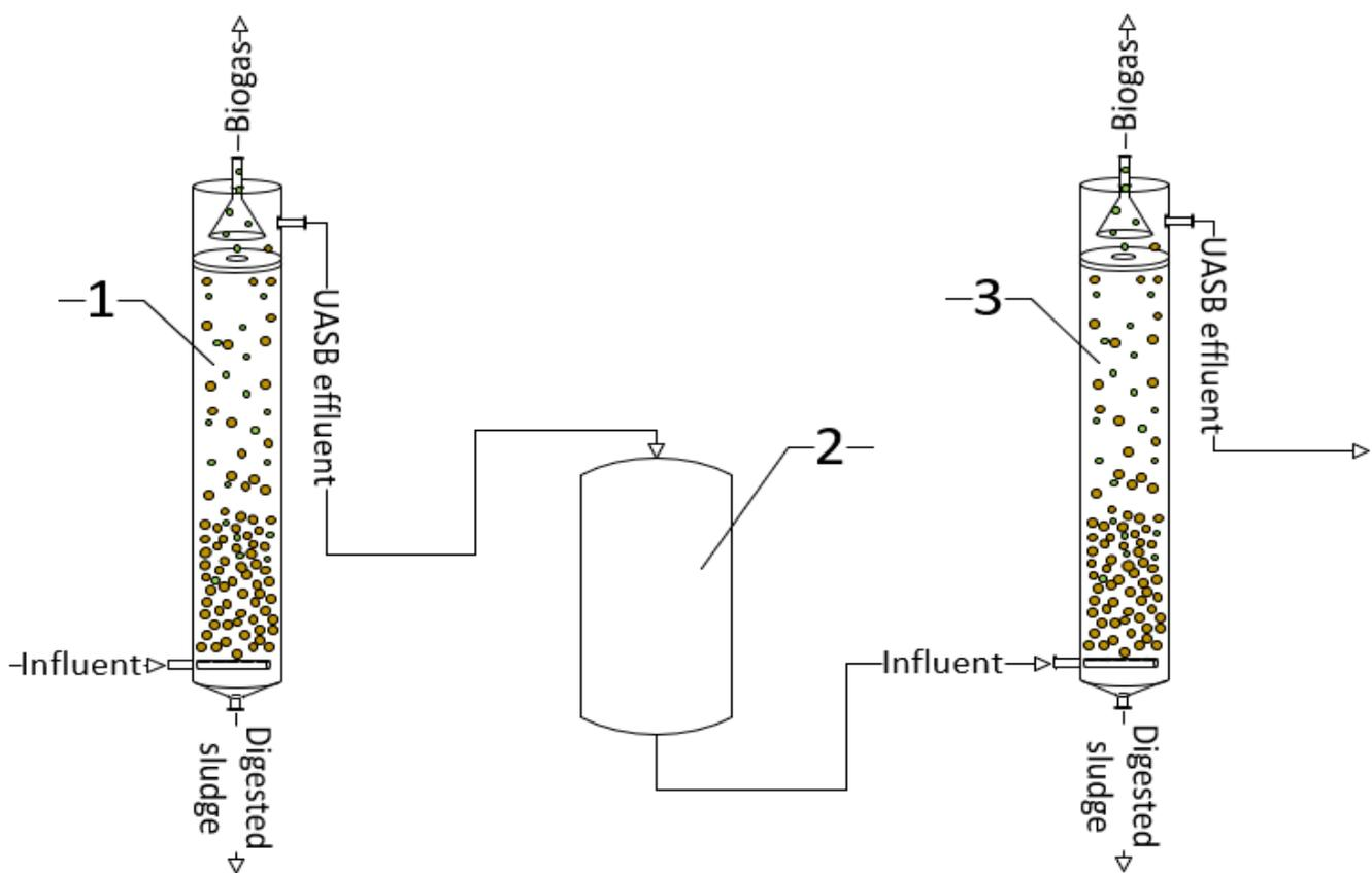
**Figure 10.** Simplified diagram of two-staged UASB system: (1) HUSB, (2) HUSB effluent tank, and (3) MUSB; based on [122].
