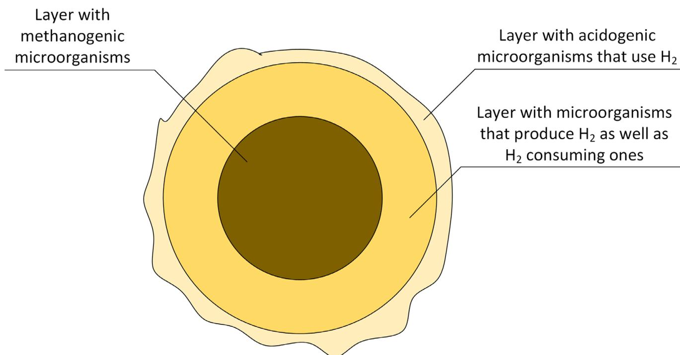
**Figure 3.** The structure of UASB granules; based on [55].
