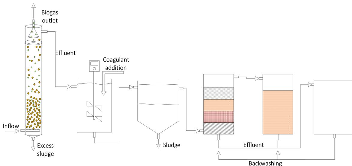
**Figure 12.** A typical process scheme of the UASB-DF system; based on [101,135].
