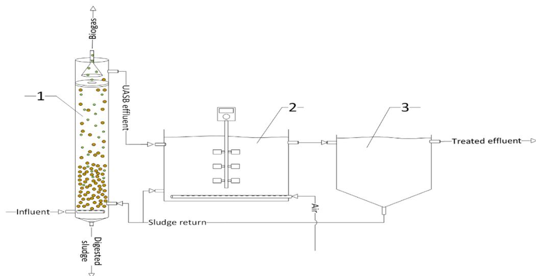
**Figure 6.** A diagram of the UASB-AS system: (1) a UASB reactor, (2) an aeration tank, and (3) a secondary clarifier; based on [18].
