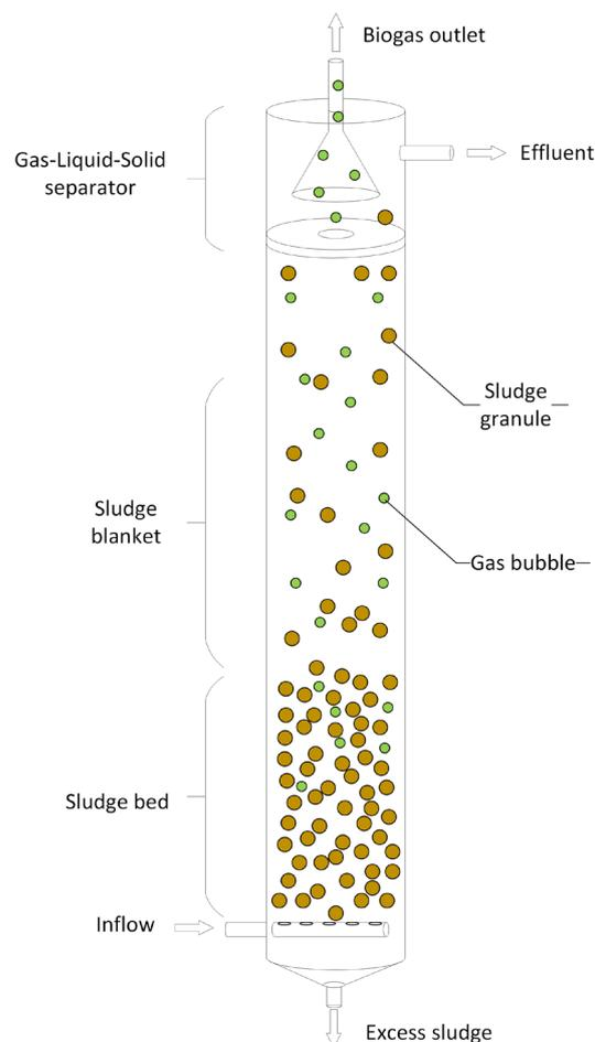
**Figure 4.** Simplified diagram of UASB reactor; based on [18,54].
