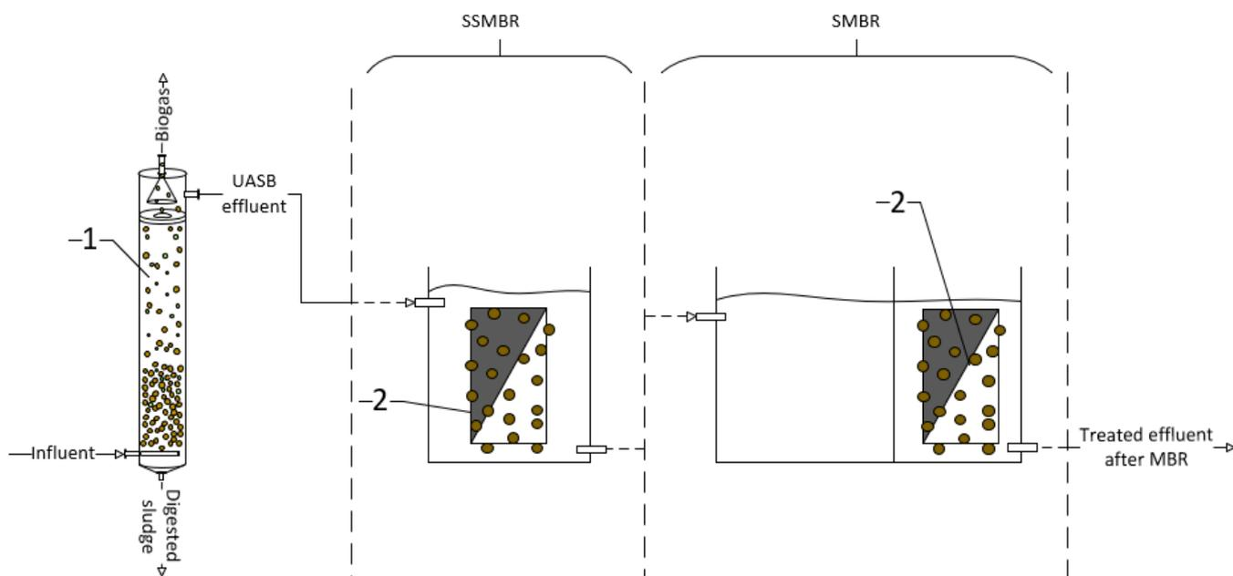
**Figure 11.** Simplified diagram of UASB-MBR hybrid system: (1) UASB and (2) membrane unit; based on [128,129].
