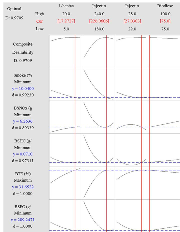
Figure 4. RSM optimization chart for engine performance and exhaust emissions.
