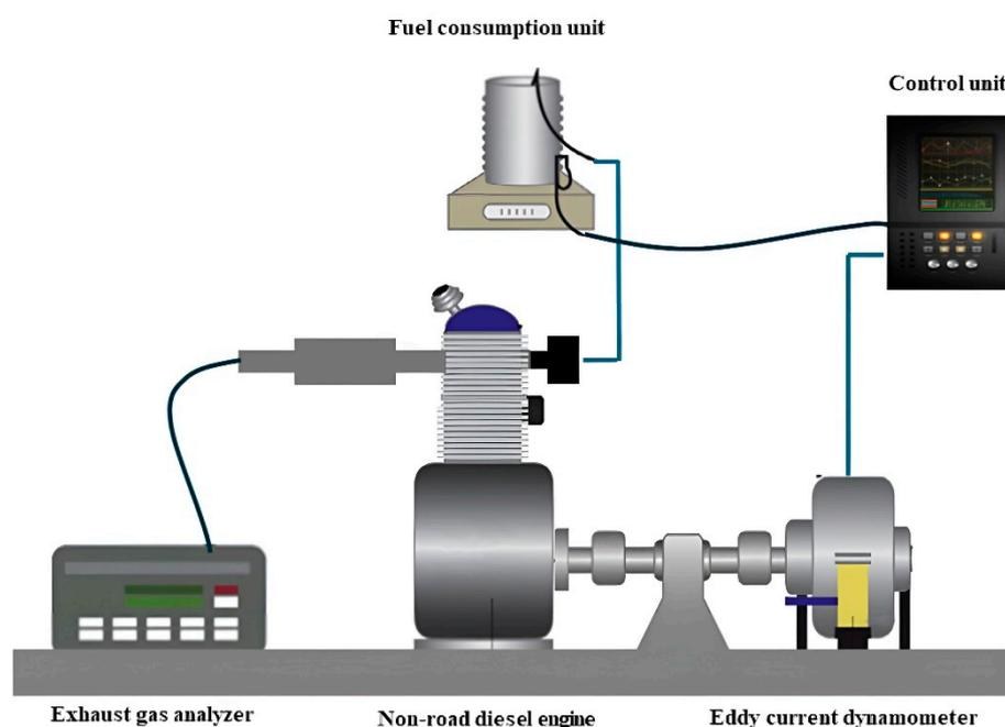
**Figure 1.** Schematic view of the experimental system.
