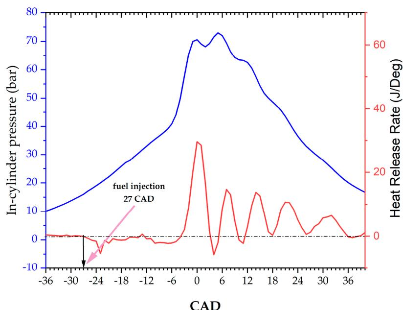
**Figure 5.** In-cylinder pressure and heat release rate curves for injection advance verification.
