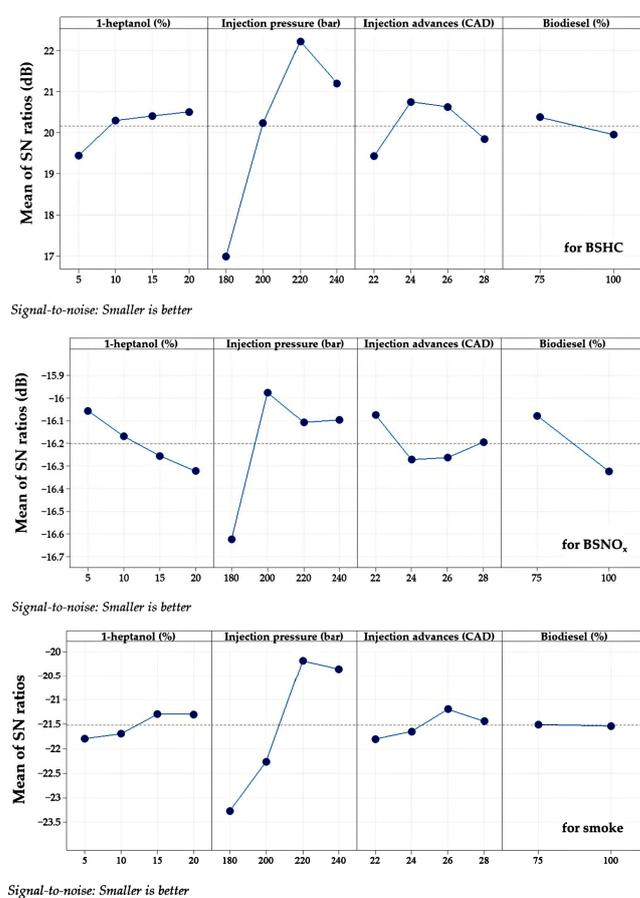
Figure 3. Main effect plots according to means of S/N ratios for exhaust emissions.
