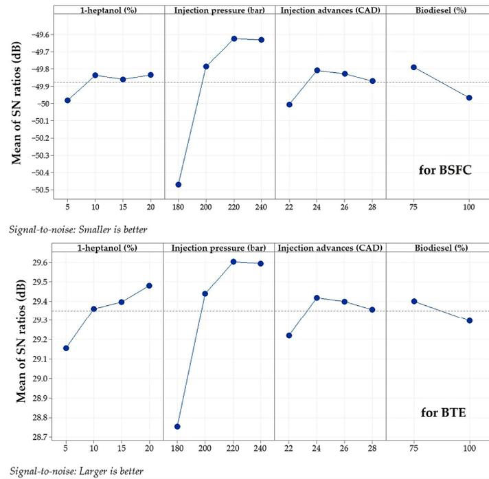
Figure 2. Main effect plots according to the means of S/N ratios for engine performances.
