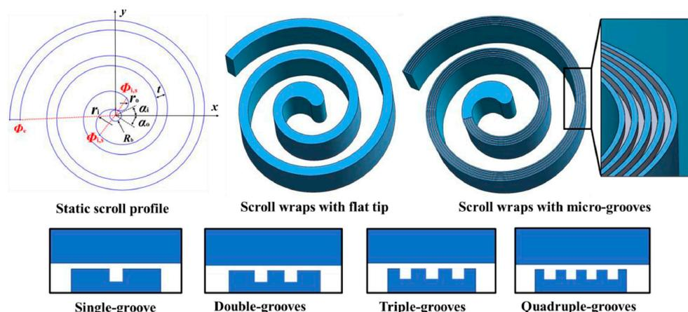
Figure 13. Micro-groove schemes proposed by Zheng [30].
