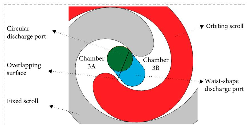
**Figure 12.** Circular and waist-shaped discharge port proposed by Song [97].
