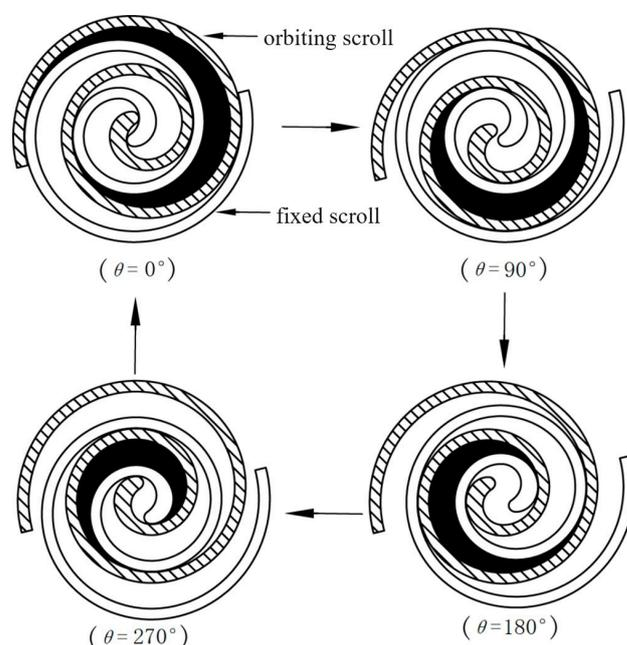
**Figure 1.** Working process of a scroll compressor.
