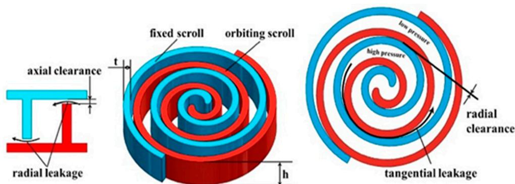
Figure 7. Scroll compressor leakage model devised by Li [58].
