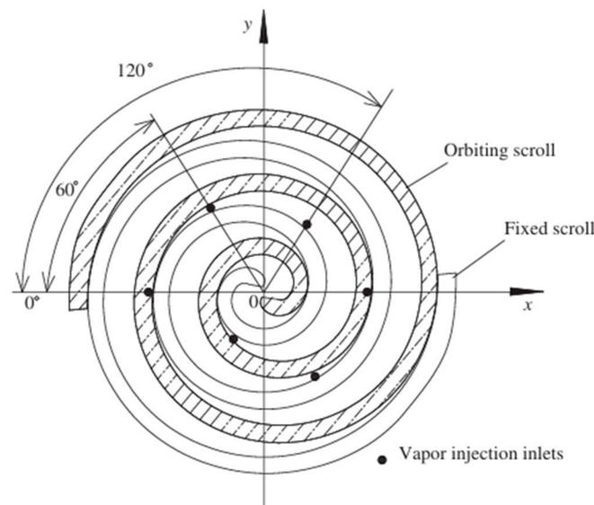
**Figure 8.** Position of scroll disk and vapor injection ports by Xu [68].
