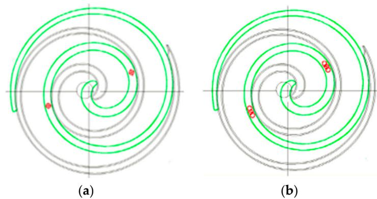
Figure 9. Two different injection ports [70]. (a) Single porthole; (b) three interlinked portholes.
