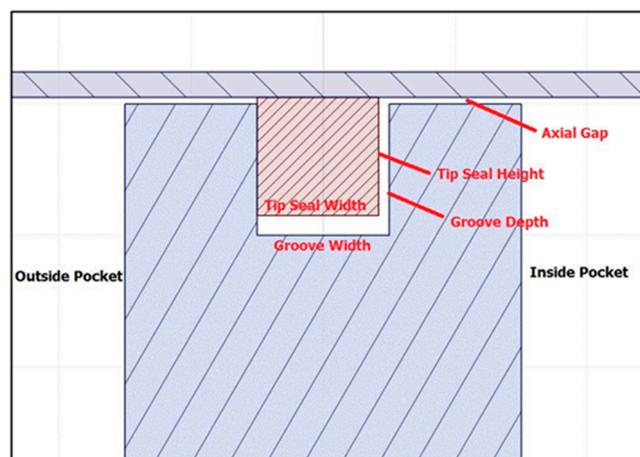
Figure 6. A typical cross-section of tip seal leakage path by Gao [54].
