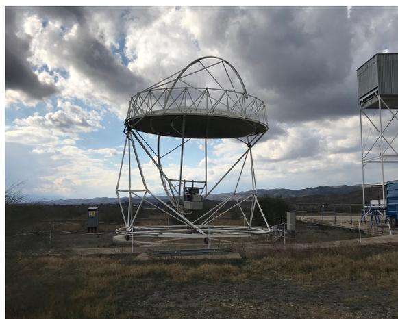
**Figure 6.** Dish/Engine system (credits © H2020 European Nexttower Project).
