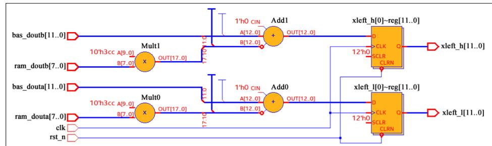
Figure 2. RTL model of right antenna update.
