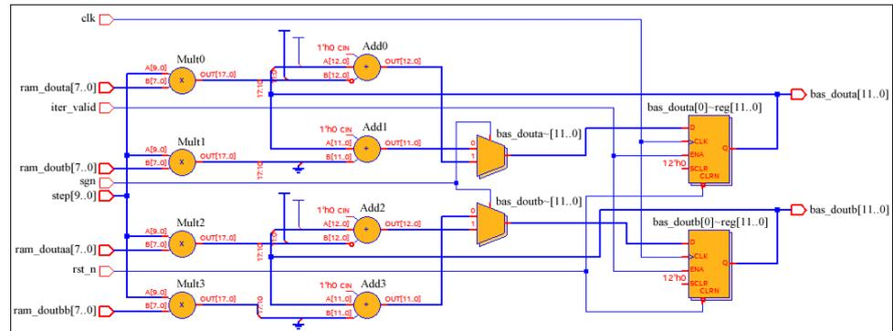
**Figure 4.** RTL model of beetle position update.
