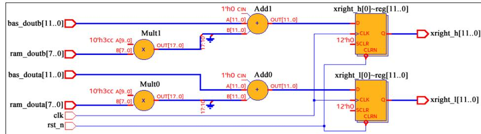
Figure 3. RTL model of left antenna update.
