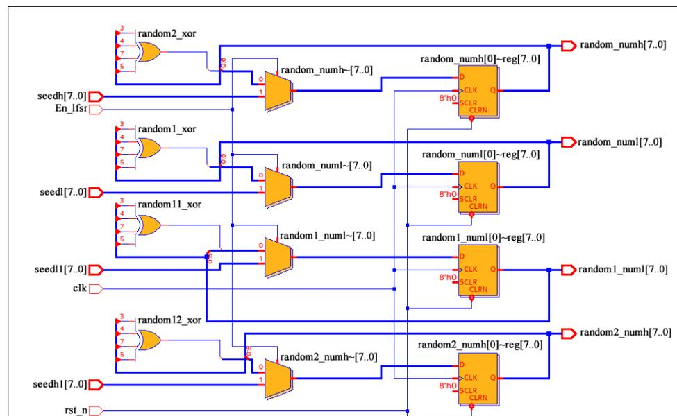
**Figure 1.** RTL model of four pseudo-random numbers from LFSR.
