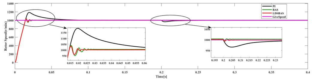
**Figure 9.** Simulation results of speed response with load transients.
