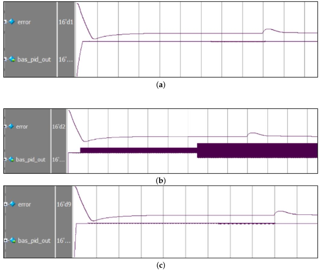
**Figure 11.** The simulation results for the PI controller with different numbers of iterations. (a) The output waveform of the PI controller with a speed loop with 200 iterations; (b) the output waveform of the PI controller with a speed loop with 100 iterations; (c) the output waveform of the PI controller with a speed loop with 50 iterations.
