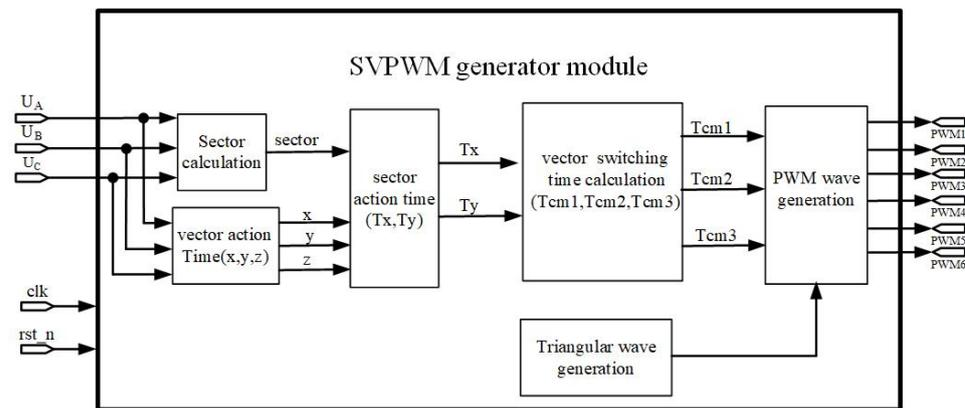
Figure 5. Three-phase SVPWM generator module.
