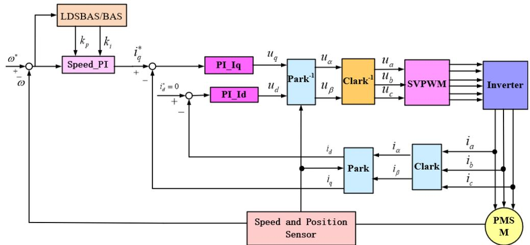
Figure 6. Block diagram of PMSM control system based on LDSBAS/BAS algorithm.
