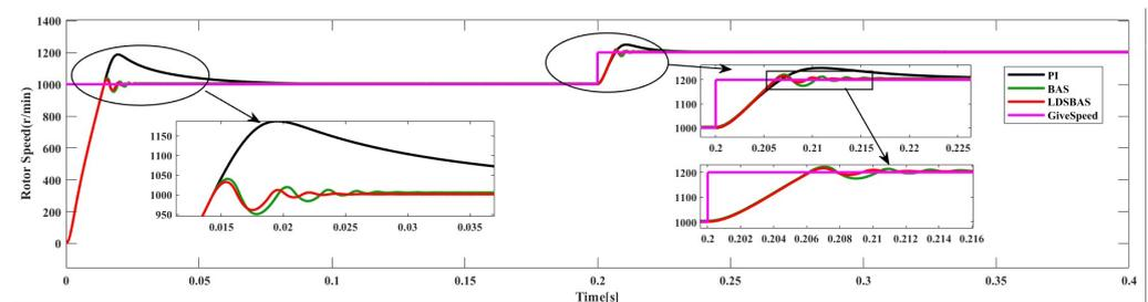
**Figure 8.** Simulation results of speed response with speed transient.
