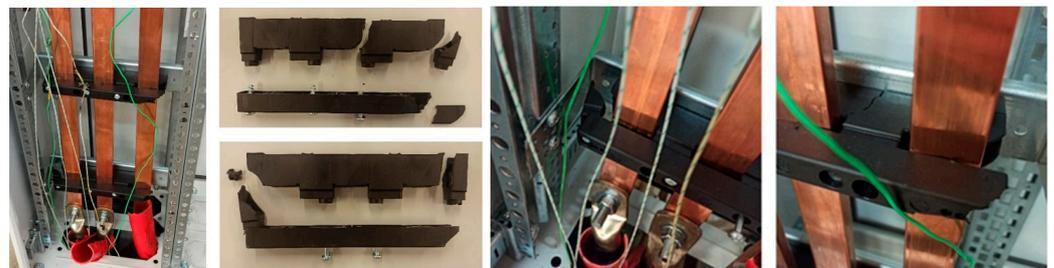
**Figure 5.** Short-circuit test results with two jumpers mounted—damaged support insulators, before dismounting and after dismounting.
