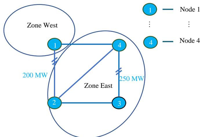
**Figure 1.** A four-node network with two capacity-constrained lines.
