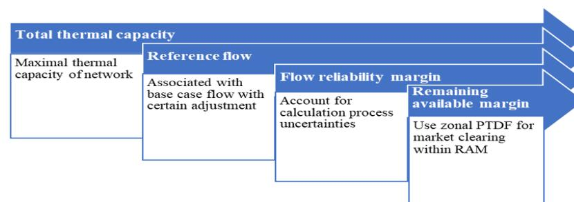
**Figure 5.** Main components of interconnection network capacity under FBMC.
