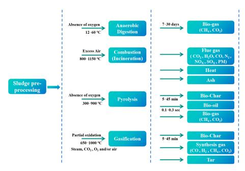
Figure 8. Energy recovery of sludge, reproduced from [1].
