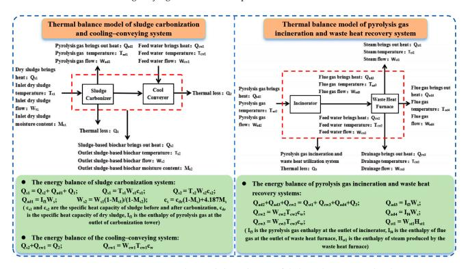
**Figure 11.** Mass and energy balance diagram of sludge carbonization and cooling–conveying system, and pyrolysis gas incineration and waste heat utilization system, reproduced from [123].
