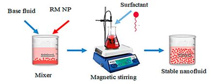
Figure 15. Preparation of RM-based nanofluids [134].
