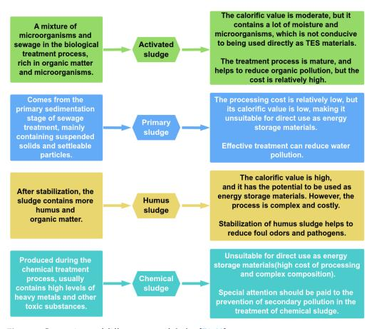
Figure 5. Comparisons of different types of sludge [74–80].
