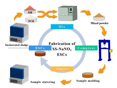
Figure 14. Production of SS-NaNO<sub>3</sub> ESCs, reproduced from [62].
