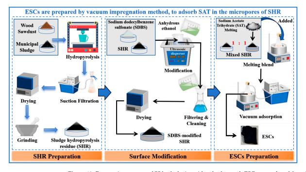
Figure 12. Preparation process of SS hydrolysis residue–hydrate salt ESCs, reproduced from [129].
