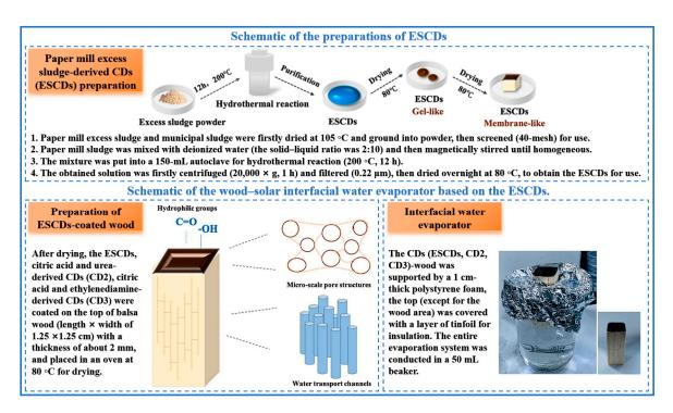
**Figure 13.** Schematic diagram of the preparation of photothermal materials and wood–solar interfacial water evaporator, reproduced from [130].
