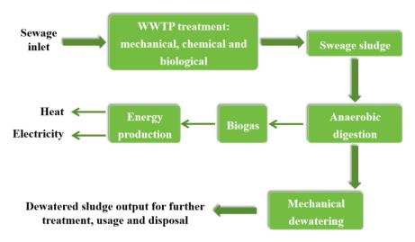
Figure 9. Flow diagram of sewage sludge treatment, reproduced from [122].
