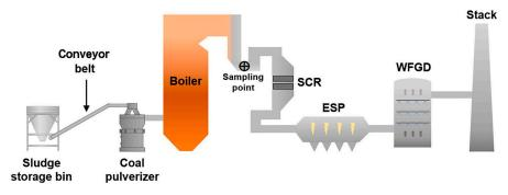
Figure 10. Flow diagram of SS for combustion power generation [121].
